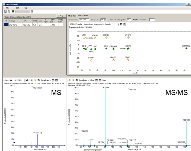
Figure 5. Formula Finder software to empirically calculate the formula of the molecular ion and fragment ions of the unexpected environmental pollutant (192 Da at 7.7min)
