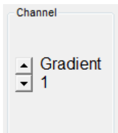
Figure 2-1 Channel Selection Controls for Eksigent Control Software
