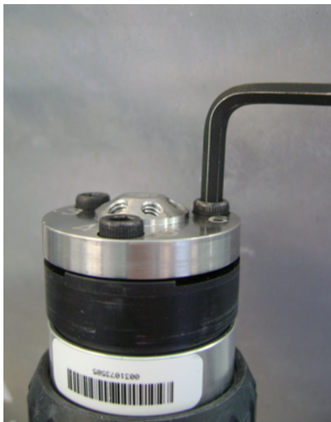
Figure 9-18 Remove the Screws in the Valve Stator
