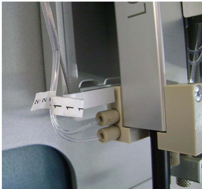
Figure 9-38 LCMS Tool Tubing, Front of System
