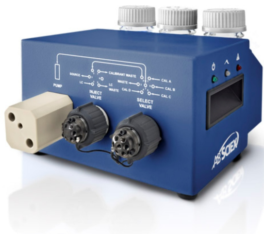
Figure 2. The Calibrant Delivery System (CDS). The CDS can accommodate up to four different solutions for calibration and tuning. Automatic external mass calibration is performed without operator intervention during sample acquisition.
