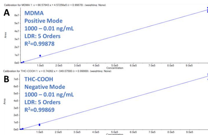
Figure 1. High Linear Dynamic Range Observed in Both Positive and Negative Modes Using the SCIEX Triple Quad 5500+ System.
