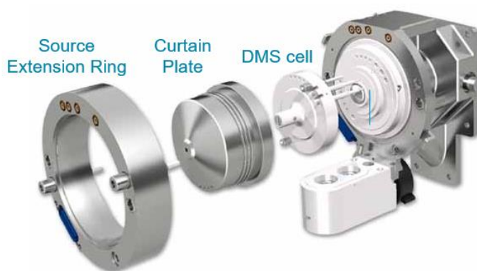
Figure 1. SelexION® Technology. The DMS interface is directly coupled to the orifice plate. A modified curtain plate accommodates the DMS cell which can be easily installed and removed without the use of any tools and without venting the system. The source extension ring enables use of the standard SCIEX sources.
