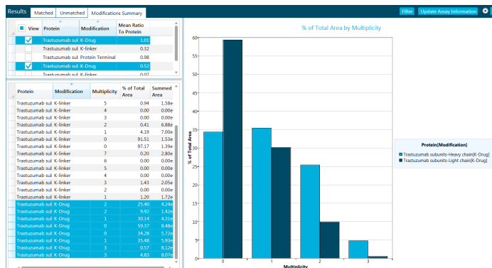
Figure 9: DAR calculations from BioPharmaView for light and heavy chain deglycosylated. Light chain shows a DAR ratio of 0.52 and the heavy chain shows a DAR of 1.01.
