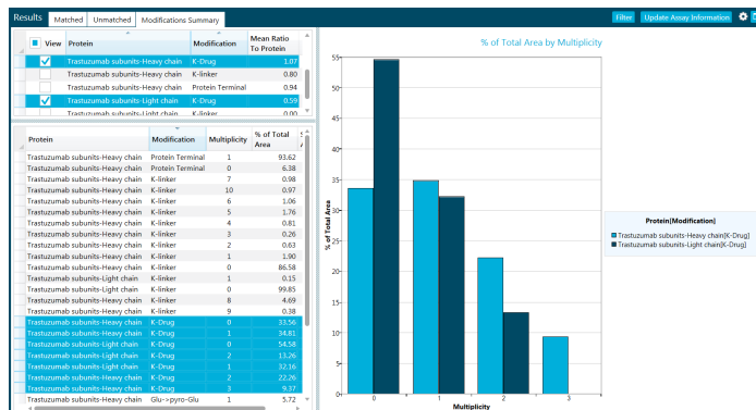
Figure 3 DAR calculation for the light and the heavy chain. Top left highlighted forms are the DAR ratios for the light (0.59) and heavy (1.07) chain.
