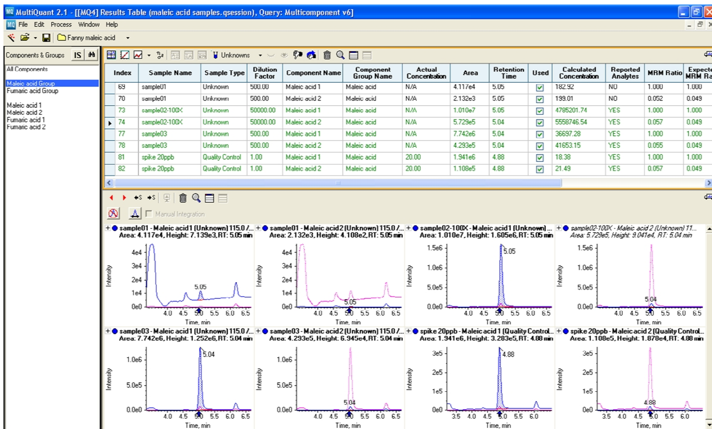
Figure 3. Results for maleic acid in different food samples, the 'Multicomponent' query in MultiQuant™ software was used to identify target analytes based on their MRM ratio
