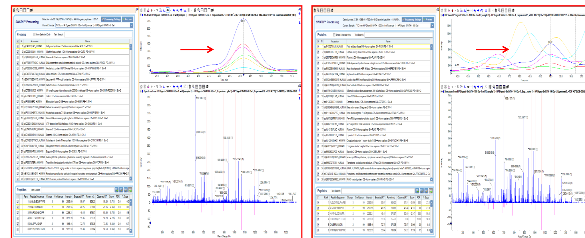
Comparative extracted ion chromatograms (XICs) of fragment ions of the peptide data acquired using 6 Da (A) and 100 Da (B) Q1 isolation window widths respectively
