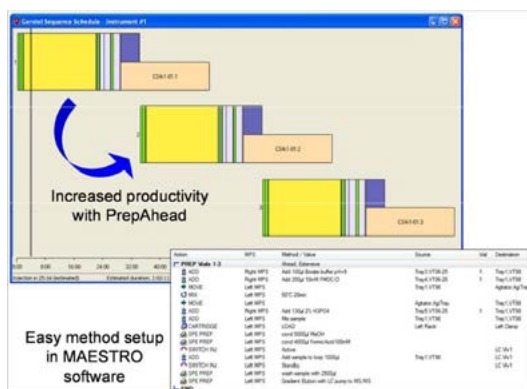
Figure 3a. Sequence of scheduled events in the Maestro software for online SPE: green - adding buffer and FMOC-Cl, yellow - derivatization, light blue - online SPE, orange LC-MS/MS analysis, dark blue washing of the autosampler, the PrepAhead function increases productivity by simultaneously preparing the following sample while perming LC-MS/MS analysis of the previous sample
