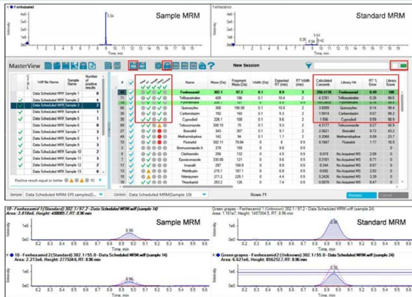
Data example: Identification of Carbendazim, Cyprodinil, Fenhexamid, Pyrimethanil, Quinoxifen, and Trifloxystrobin in a grapes sample (QuEChERS extract 10x diluted), however, only Fenhexamid and Pyrimethanil were present at a concentration higher than 10 µg/kg Confirmation of Fenhexamid using a second analysis and automatic ion ratio calculation in MultiQuant™ software
