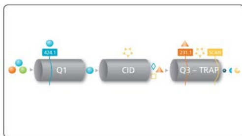
Figure 1. MRM 3 for Quantitative Analysis by LC-MS. Analyte ion is first selected in the Q1 quadrupole, then fragmented in Q2 collision cell. Fragment ions are trapped then isolated in the linear ion trap, followed by excitation to perform the second fragmentation step. Second generation product ions are scanned out to the detector.
