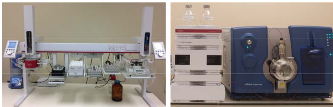
Figure 1. The GERSTEL MPS 2XL equipped with a CF-100 dual position centrifuge, mVAP multi-evaporation station, mVORX vortex and DPX option and the SCIEX QTRAP® 4500 system
