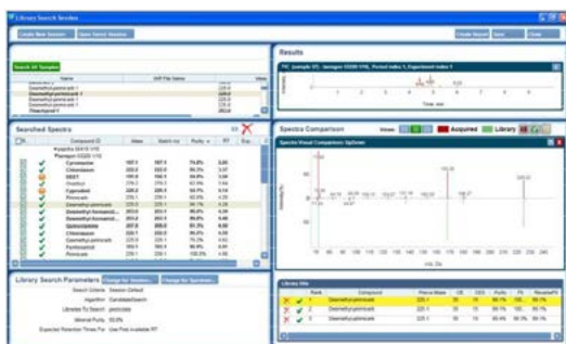
Figure 9b. Automated library identification for Desmethyl-pirimicarb detected in a paprika extract after DPX-QuEChERS LC-MS/MS
