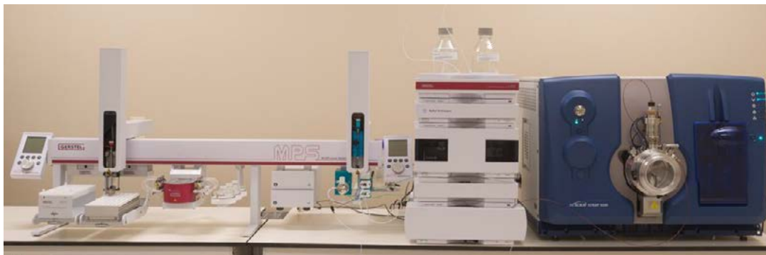
Figure 1. GERSTEL MPS 2XL with DPX option coupled to an QTRAP ® 4500 system
