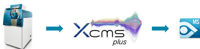
Figure 1. Workflow for Metabolic Profiling using the TripleTOF System. Data is taken from the TripleTOF 6600 system and processed through XCMS Plus software for feature finding. The metabolite identifications are confirmed by taking the metabolites of interest and passing them through the accurate mass metabolite library in MasterView™ Software.
