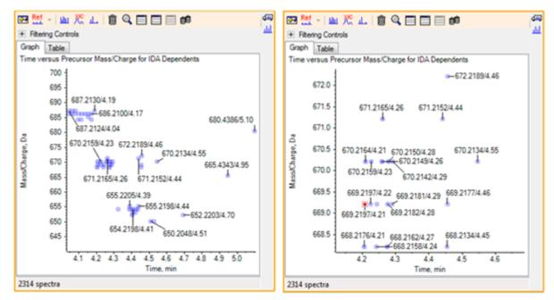
7. Select the first of the 669.2197 peaks (shown as an asterisk in the right panel above) and then click the **Displays an XIC for selection** icon to show the XIC for this precursor mass in the survey scan.
