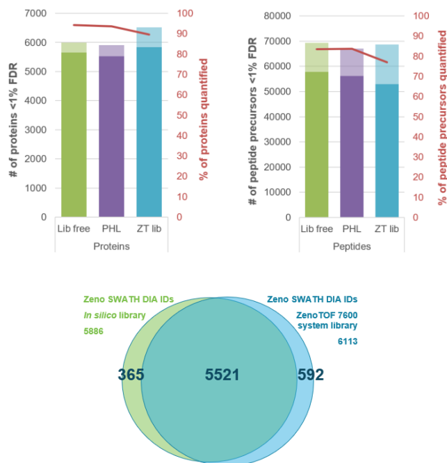
Figure 3. Comparing protein identification results from 3 different library approaches. The nanoflow Zeno SWATH DIA data from the 100 ng sample load was processed using 3 different libraries (Lib Free, using an in silico library from a FASTA file; PHL, Pan Human library; ZT Lib, large library from a Zeno DDA dataset). (Top) The numbers of proteins identified at <1% FDR (transparent) and quantified at <20% CV (solid) were measured. (Bottom) The proteins identified using the library-free approach or the ZenoTOF 7600 library were compared. Very good overlap was observed in the detected proteins.
