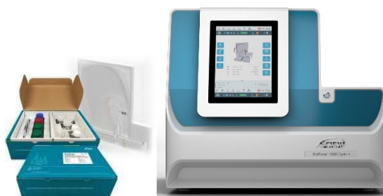
Figure 1. The BioPhase 8800 System equipped with consumable/reagent kits, LIF and UV detectors
