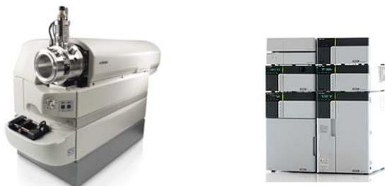
Experiments were performed using a 3200 QTRAP<sup>®</sup> LC/MS/MS System (left) and a Shimadzu Prominence HPLC System (right).
