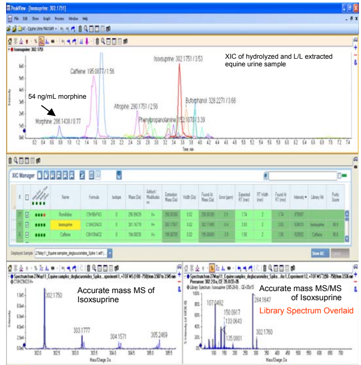
Figure 4. The drugs Atropine, Caffeine, Isoxsuprine, Morphine, Indapamide, Diclofenac, Meclofenamic Acid and Clenbuterol were identified using retention time, mass error, isotope pattern and confirmed with MS/MS library matches. Other spiked drugs that were not in the library were identified by retention time, mass error and isotope pattern. All drugs were also quantified; the example given is morphine (54 ng/mL).
