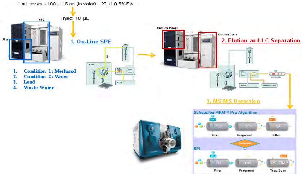
Figure 2. Graphical representation of the automated On-Line SPE LC-MS/MS workflow with Spark Holland PICO and SCIEX QTRAP® 4500 LC-MS/MS System
