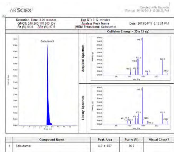
**Figure 10.** The Cliquid® Software was used to automatically generate a report after automated acquisition, data processing and library searching. An extract from the report is shown, showing the integrated MRM signal of Salbutamol and the comparison of the acquired EPI spectrum and the spectrum from the library.
