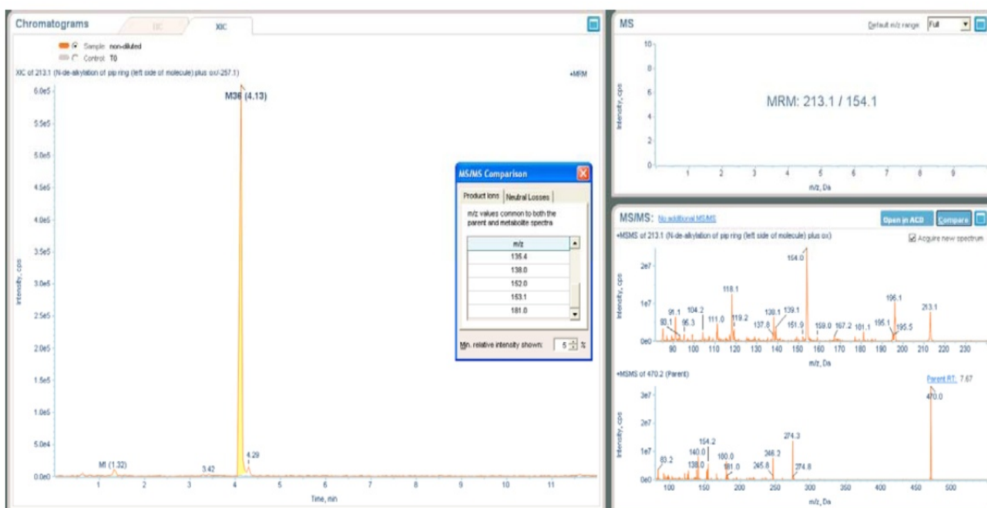
Figure 5. N-dealkylation of the chlorine containing ring on the left half of the molecule plus addition of an oxidation and dehydrogenation. The QTRAP ® 5500 System LIT sensitivity provides superior fragmentation detail.
