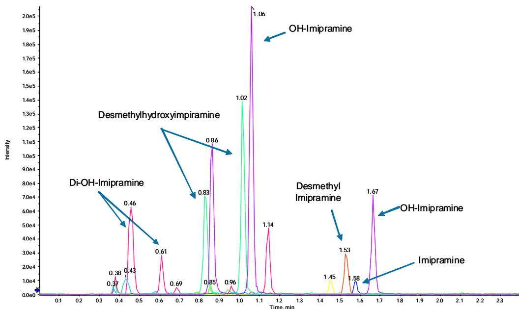
**Figure 6. Broad Coverage for Phase I Metabolites.** Overlay of accurate mass XIC's for imipramine incubation at 5 minutes. A wide range of imipramine Phase I metabolites were easily detected using a completely generic TOF MS IDA method in under 2.5 minutes.
