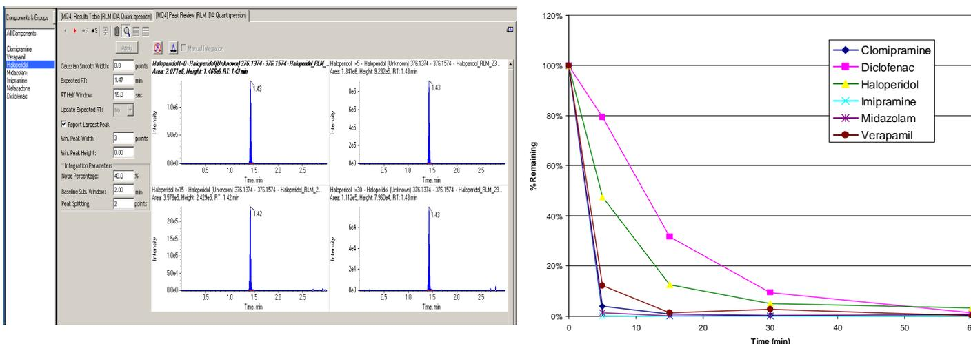
**Figure 3. Data Processing in MultiQuant™ Software.** (a) TOF MS data was easily processed for multiple analytes to obtain quantitative data. (b) Metabolic stability profiles of 6 common substrates incubated at 1 μM and analyzed using TOF MS with IDA triggered MS/MS.
