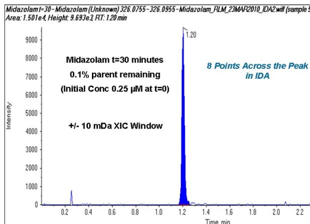
**Figure 4. Sensitivity and Speed.** The 30 minutes time point from Midazolam microsomal incubation with 0.1% of parent remaining (0.8 pg on column). Analyte is easily detected in TOF MS IDA mode with 8 data points. Each point consists of a survey scan and two MS/MS dependent scans.
