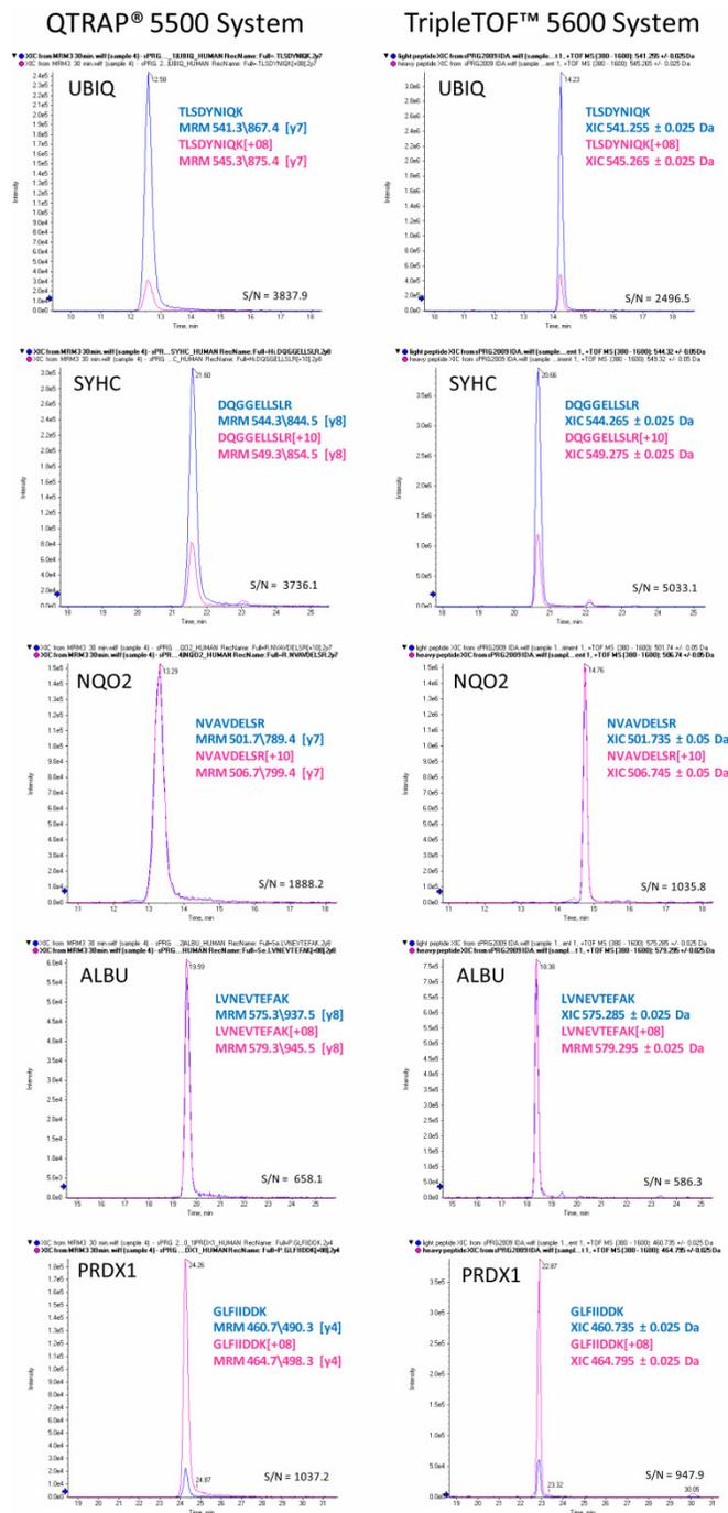
**Figure 4. Comparing Quantitation Quality.** Shown is a comparison between the quantitation obtained from extracted ion chromatograms (XICs) from TOF MS on the TripleTOF™ System and the best MRM transition acquired on the QTRAP® 5500 system for the light [blue trace] and heavy [pink trace] labeled peptide set for each target protein.
