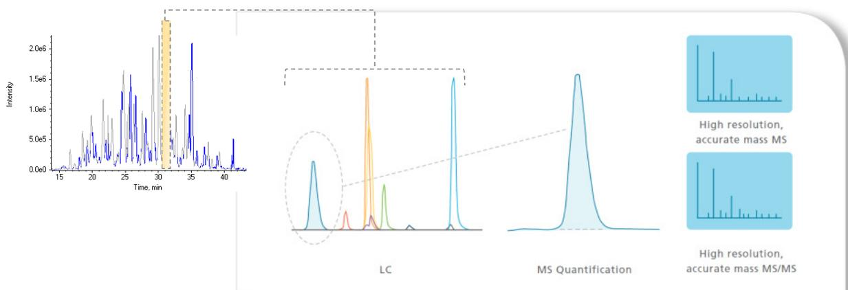
**Figure 1. Profile Workflow for Simultaneous Protein Identification and High Resolution MS Peptide Quantification.** From an LCMS separation, many features are resolved in the MS data, especially when using a high resolution TOF MS scan. In this workflow, the quantitative information for many of the peptides identified from the high resolution and high mass accuracy MS/MS data can be extracted from the accompanying MS data.
