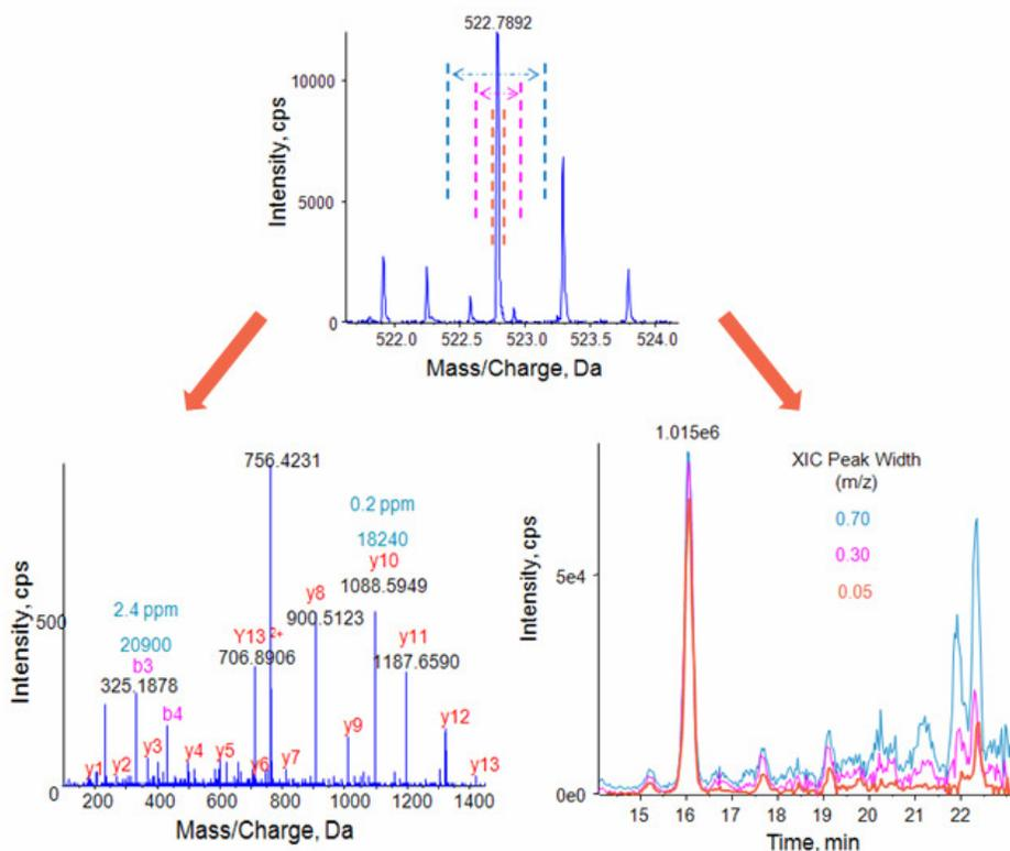
**Figure 2. High Resolution Extracted Ion Chromatograms (XIC).** Because of the high resolution TOF MS data and the high mass accuracy that is easily attained across extended LCMS operation, it is possible to generate MS XICs at high resolution for highest specificity. In the same run, high quality MS/MS spectra for identification are generated.
