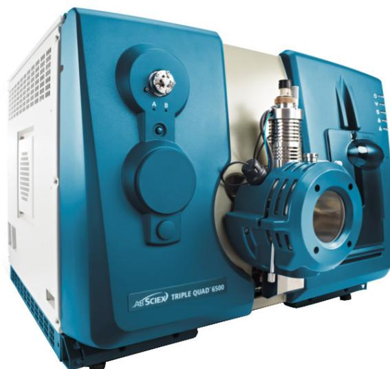
The SCIEX Triple Quad™ 6500 tandem mass spectrometer, featuring IonDrive™ technology, delivers ultra-sensitive detection enabling the quantitation of trace levels of steroid hormones in biological fluids.
