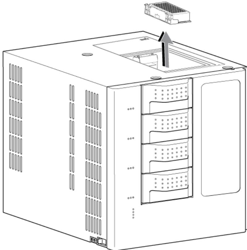
7. If the fallen rack is a condensation-prevention rack, then return it to the condensation-prevention rack box. If it is a normal rack, then return it to an empty stack.
