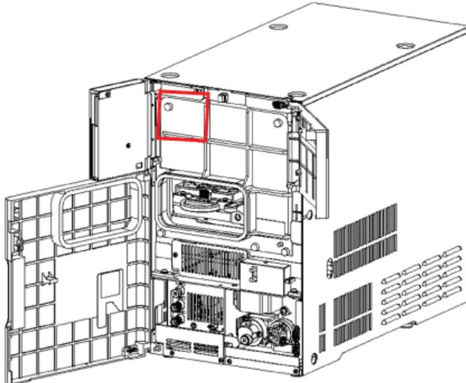
12. Loosen one screw at the bottom right of the Z mount.
