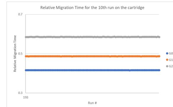
Figure 7. Relative migration time behavior observed across the cartridge run life.
