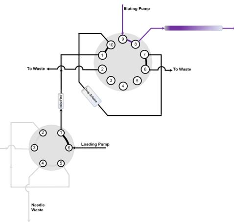
Figure 1. Trap-and-Elute Workflow Flow Diagram
