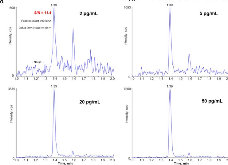
Figure 3. Low Level MRM Chromatograms of Exenatide in Crashed Plasma Using Microflow LC Trap-and-Elute Workflow
