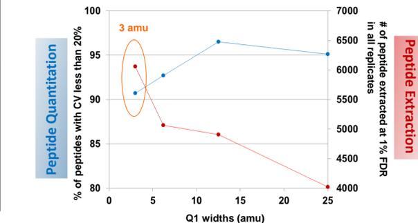
**Figure 4.** A summarized illustration of the impact of Q1 isolation window sizes on the peptide extraction and quantitation. It clearly demonstrates the improved peptide extraction with smaller Q1 widths applied without compromising the quantitative reproducibility.
