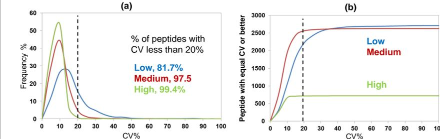
**Figure 3.** (a) The dependence of CV% distribution on the peptide abundances spanning over ~4 orders of magnitude. The peptides are sorted by intensities into three bands, as presented with blue, red and green traces corresponding to low (< 10<sup>5</sup>), medium (10<sup>5</sup>-10<sup>6</sup>) and high (> 10<sup>6</sup>) intensities respectively. (b) Cumulative plot of peptides vs. CV% in three intensity bands, showing the numbers of peptides in each intensity band.
