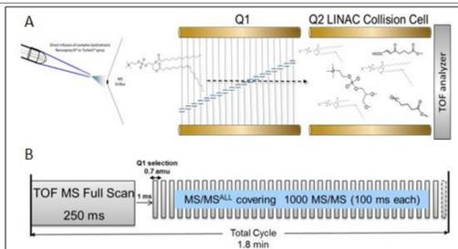
**Figure 2. Infusion MS/MS<sup>all</sup> Workflow.** Lipid precursors are selected at unit resolution in Q1, fragmented, and all product ions are detected simultaneously (A). Using infusion MS/MS<sup>all</sup> method, which is automated collection of TOF MS and TOF MS/MS of all lipids via step-wise sampling of all precursor ions selected at unit resolution (B). This acquisition requires 1.8 min to generate a comprehensive dataset.
