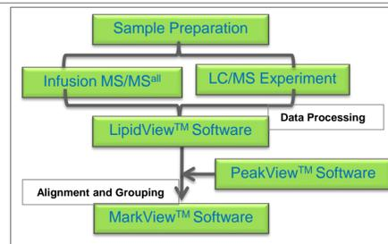
**Figure 1. Lipid Profiling Workflow.** Step 1. Data acquisition using infusion MS/MS<sup>all</sup> and LC/MS methods. Step 2. Lipid molecular species identification and quantitation using LipidView™ software. Step 3. Grouping difference Compare using MarkerView™ software.
