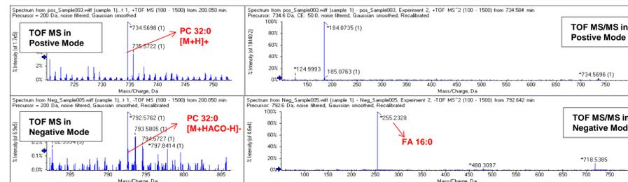
**Figure 6. By combining TOF MS/MS in positive and negative mode, the specific lipids can be identified in PeakView™ Software.**
