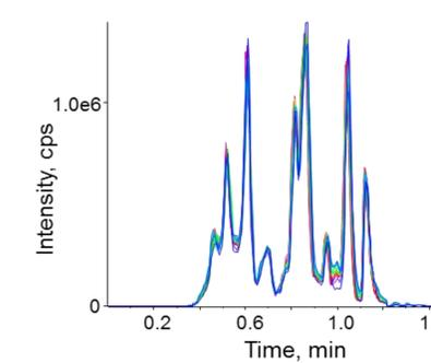
**Figure 3.** TIC Overlay of 20 replicate injections. Average CV per MRM is 7.7%
