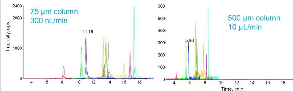
**Figure 1. Comparison of the MRM Traces at the Lowest and Highest Flow Rates.** The MRM chromatogram for the 10 peptides from the 75  $\mu$ m ID column was obtained using a 15 min linear gradient, peptides are observed from 8 – 18 mins (top). At the higher flow rates, faster gradients can be used. Analyzing the same peptides on a 500  $\mu$ m ID column shows a small decrease in sensitivity but an increase in throughput (7 minute linear gradient). However equivalent resolving power was obtained.
