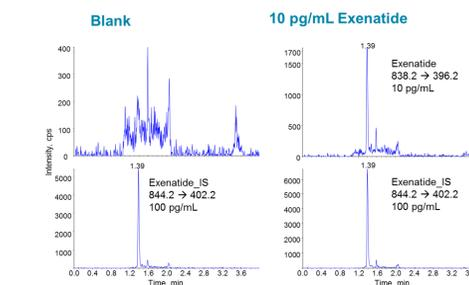
**Figure 6.** MRM chromatogram for matrix blank with IS and 10 pg/mL Exanatide showing minimal carry-over.
