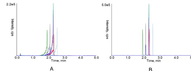
Figure 2. Comparison of the chromatography obtained in standard microLC injection configuration (A) and ODR configurations (B). 1  $\mu$ L of triazenes mix in 100% methanol was injected for both configurations.
