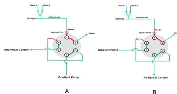
Figure 1. Injection valve in inject position, left is standard configuration and right is the Online-Diluting-and-Refocusing (ODR) configuration
