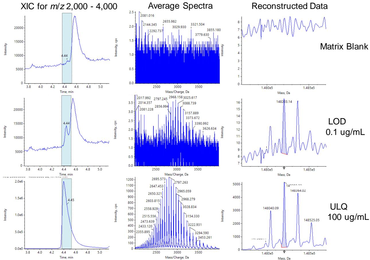
**Figure 5: Overview of Quantification Results from SCIEX OS Software.** XIC, average spectra and reconstructed data information for the matrix blank, the lowest concentration and the highest concentration used for quantification. The analyte protein is eluting at 4.44 min, the additional peak being visible in the matrix blank and the LOD at 4.55 min is related to the elution of matrix proteins.
