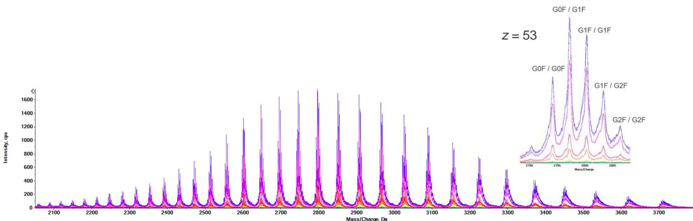
**Figure 2: TOF-MS Raw data for Replicate Injections of Different Concentrations of NIST mAb Analyte in Processed Plasma Matrix. Upper right hand side: Zoom into highest abundant charge state  $z = 53$  with indication of the different glycoforms of the antibody sample.**
