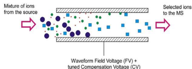
**Figure 2. Principle of differential ion mobility spectrometry (DMS).** As the mixture of ions enters the drift tube, they are separated according to differences in each individual molecule's size, shape, and charge. An optimized combination of separation voltage (SV or waveform field voltage, FV) and compensation voltage (CV or COV) separates the analyte from background ions.
