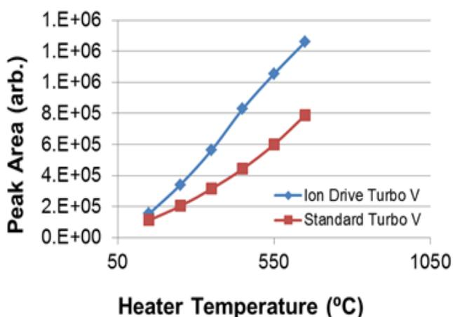
**Figure 2: Comparing Peak Areas Between Sources.** Measured peak area for Lidocaine using the Turbo V (red) and IonDrive Turbo V (blue) sources. All instrumental variables held constant other than swapping sources on a QTRAP 6500 System.
