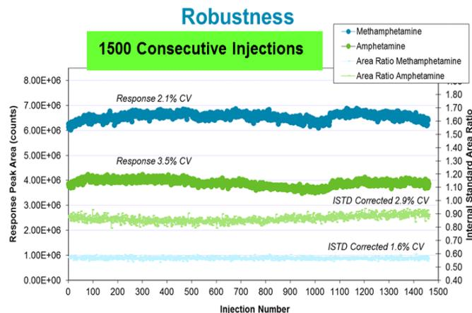
**Figure 4. Robustness of IonDrive Source.** 1500 consecutive injections of methamphetamine and amphetamine in protein precipitated rat plasma (no divert valve) continuously over 3 days. The peak area counts and peak area ratio for both compounds were stable with % CV <3.5.
