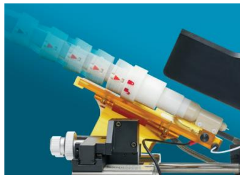
Figure 6. Mounting of the OptiMS Cartridge on the NanoSpray III Source. Remove the union mounting rail and the OptiMS cartridge tip easily slides into place.
