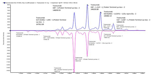
**Figure 5: Comparison of glycoforms and intensities of the reconstructed spectra of the two lots of trastuzumab. Lot 1 in blue and Lot 2 in pink.**
