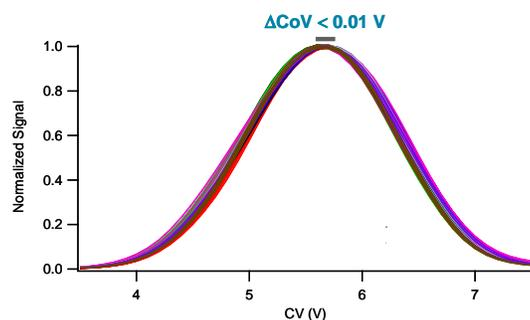
**Figure 5. High Stability of Compensation Voltage.** CoV stability is a key requirement for reproducible bioanalytical quantification with DMS. CoV remained within 0.01V when measured repeatedly over 24 hours demonstrating excellent stability.
