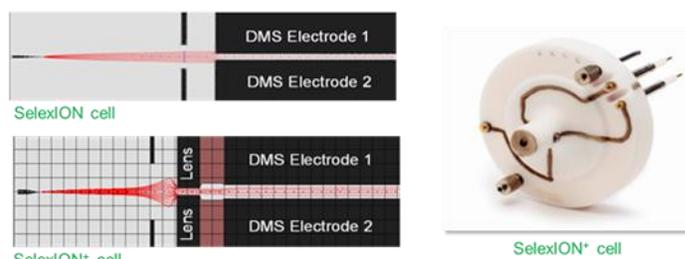
Figure 3. Comparison of SelexION and SelexION+ Technology. The addition of the jet injector to the ion mobility cell improves ion transmission by 2 fold without loss in selectivity or resolution compared with the original SelexION technology.
