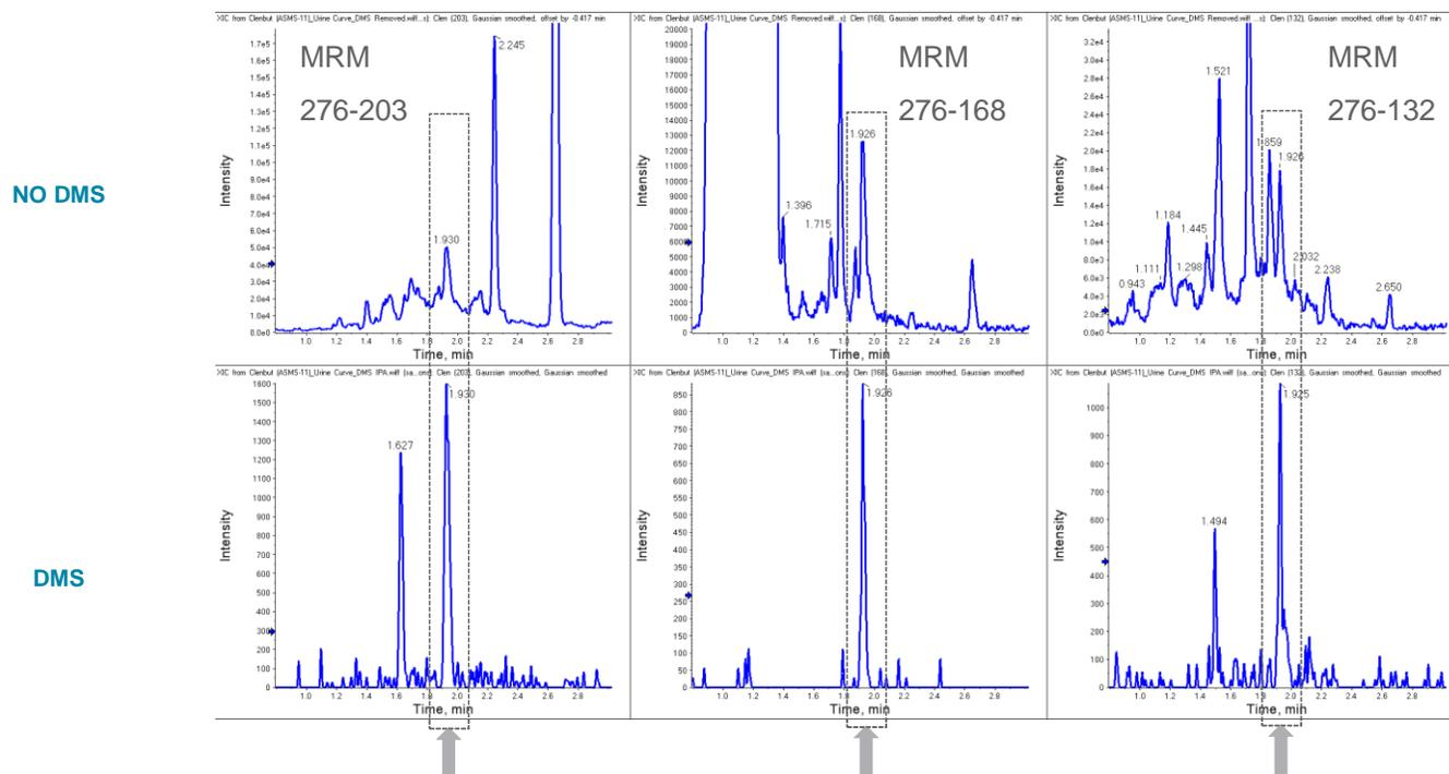
**Figure 4. Analysis of Clenbuterol in Urine.** This assay suffers from matrix interferences in all three MRM channels (top). Using SelexION Technology with isopropanol as a chemical modifier resulted in the reduction or elimination of interferences in all three MRM channels (bottom).
