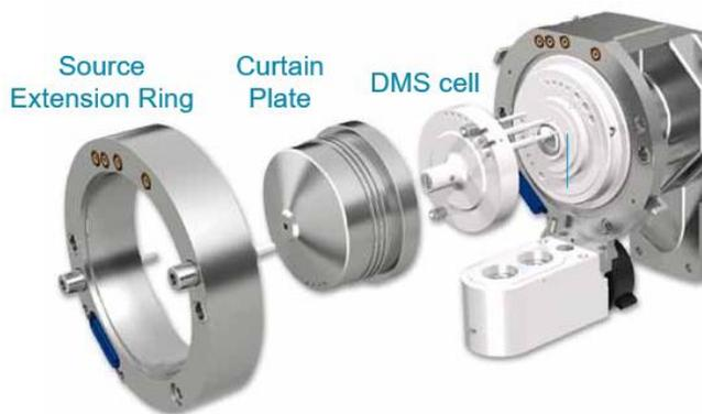
**Figure 1. SelexION<sup>®</sup> Technology.** The DMS interface is directly coupled to the orifice plate. A modified curtain plate accommodates the DMS cell which can be easily installed and removed without the use of any tools and without venting the system. The source extension ring enables use of the standard SCIEX sources.
