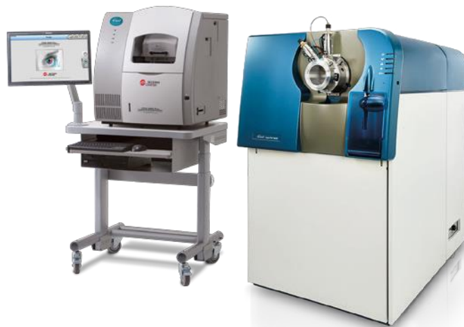
CESI 8000 Plus High Performance Separation Module coupled to a TripleTOF® 6600 System via a Nanospray III source, CESI adapter, and neutral-coated OptiMS capillary cartridge
