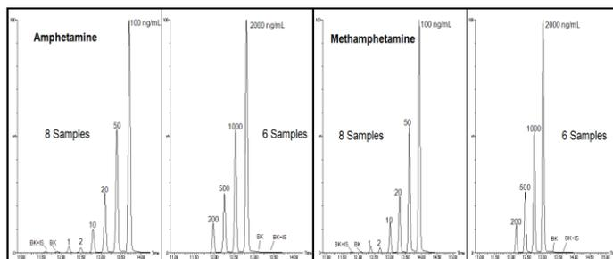
Figure 3: MSI Calibrations for Amp/Meth 8 and 6 Sample Runs
