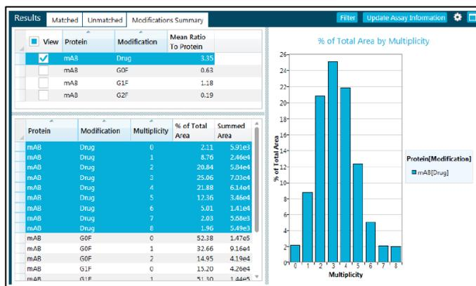
**Figure 5** Automated DAR calculations for the non-deglycosylated ADC. The reconstruction area is given as a value, and also as a percentage of the total area per each multiplicity of conjugation. The multiplicity is represented as columns and the final DAR ratio is calculated.
