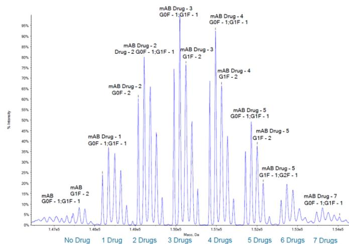
**Figure 4** BioPharmaView software reconstruction of the data presented in Figure 3 Drug load was up to 7 per antibody moiety, with all the different drug conjugations demonstrating the same glycosylation pattern of combinations of G0Fs to G2Fs.
