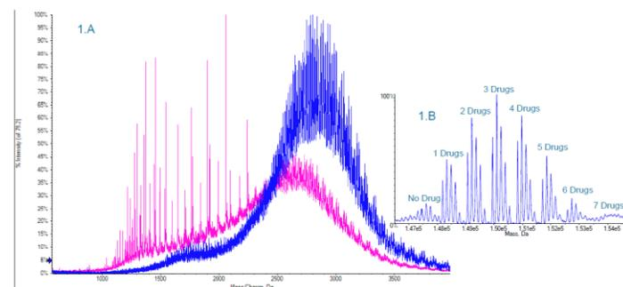
**Figure 1** (A) comparison of raw spectra from the chromatographic system 1: reverse phase separation. In Blue: spectra with SelexION® technology cell optimized for the transmission of ADC ions. In Pink: no differential mobility separation applied. (B) Reconstructed spectrum of the SelexION technology-acquired data.
