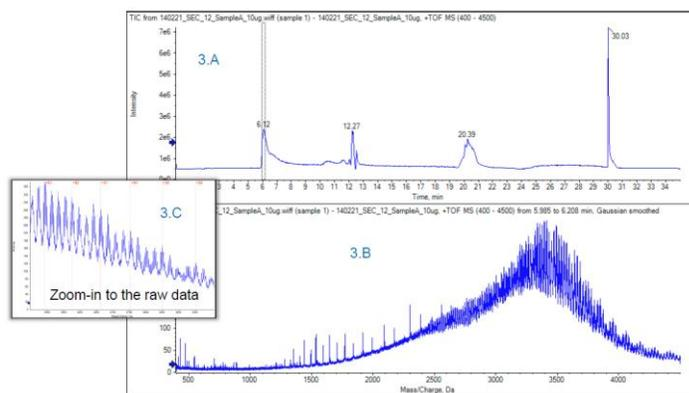
**Figure 3** Chromatographic system 2 (SEC separation) Total Ion Chromatogram (3A) and the obtained ADC raw spectrum (3B) and a zoom-in of the spectrum (3C) with the charge states highlighted
