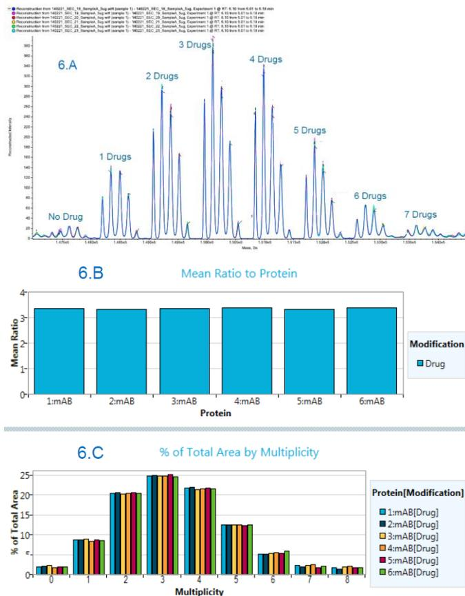
**Figure 6** Reconstruction of analysis of six injections of the non-deglycosylated ADC: (6A) the overlay of six reconstructed spectra, (6B) the DAR ratios and (6C) the multiplicity represented as columns for the six injections.
