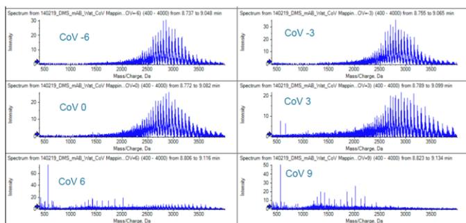
**Figure 2** Optimization of the SeleXION technology compensation voltages (CoV) on a monoclonal antibody (mAb). Panes have been marked with the applied CoV (here shown from -6 to 9). The separation voltage was optimized to 3500V. For large proteins such as mAbs, the transmission optimum was found with negative CoVs; for the smaller proteins (Ab light chain) and interferences, the transmission optimum was found with positive CoVs.
