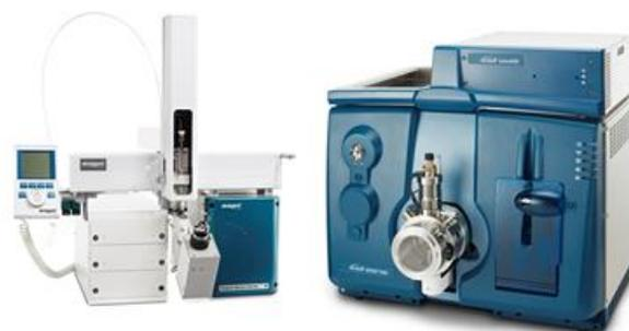
Differential mobility spectrometry (DMS) on QTRAP® systems, known as SelexION® Technology, can be used to separate peptides based on different chemical properties and can be functional in the separation of isobaric or isomeric compounds. In this study, peptides with different modification sites or types were analyzed using SelexION Technology on the QTRAP® 5500 system.
