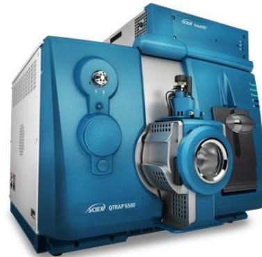
screening, confirmation and identification applications. With a QTRAP system, all of the MRM sensitivity of a QqQ is combined with a multi-functional ion trap with no compromises. Not only does this afford the highest performance for quantitative and qualitative experiments on the same instrument, it also enables new and powerful TripleTrap™ Scanning workflows that combine QqQ functionality with LIT functionality within the same experiment.
