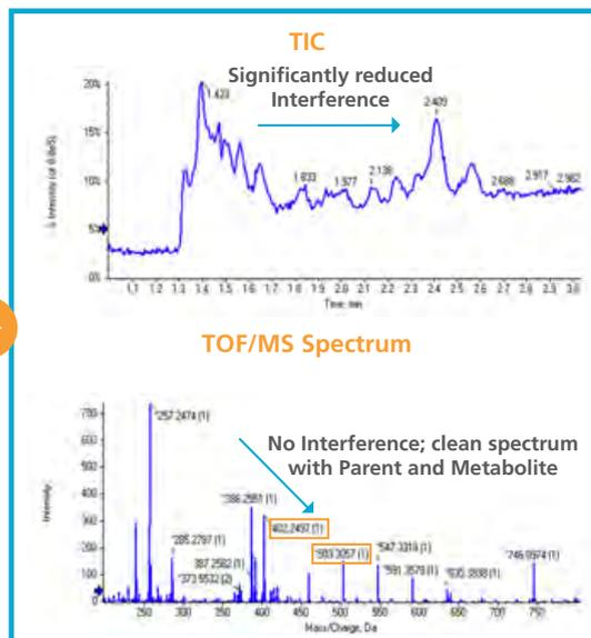
Detect the presence of metabolites that may be masked by high intensity matrix interferences by using SelexION Technology to filter out interfering ions
