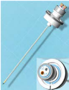
Figure 2. TwinSprayer ESI probe showing the independent inlet for LC and calibrant
