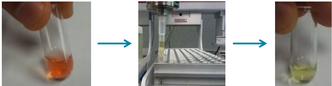
Figure 4. Schematic of the automated DPX-QuEChERS procedure, 500 µL of apple extract (left) and after DPX-QuEChERS cleanup (right)
