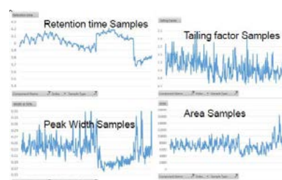
Figure 5. Reproducibility data for glyphosate IS. NofaLab method for food samples, tested over 1000 injections of extracts from fruit/veg, seeds, veg oil/fat, grains, herbs/spices, meal/fish, animal oil/fat, eggs/egg products, milk/milk products and other fatty acids.
