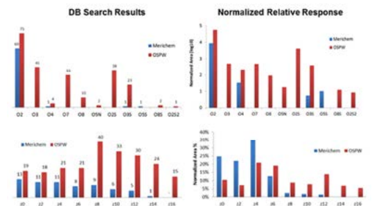
Figure 8. Evaluation of Merichem and OSPW samples as a function of the number of database-identified compounds grouped by class (left) and area response (right). Results are further broken down by compounds class (top) and z -value (bottom). Values shown above the homologue plots are the number of homologues identified during database (DB) searching. Due to the large differences in absolute response between compound classes this data was converted to a log10 scale.
