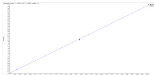
Figure 4. Glyphosate calibration standards. Linear calibration regression for glyphosate with 1/x weighting, showing r-value of 0.9997 and excellent precision for duplicate calibrators.
