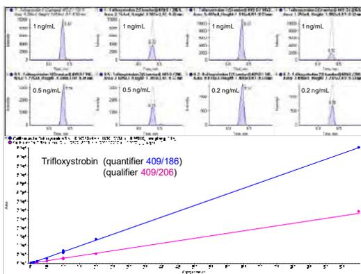
Figure 4b. Calibration lines of the quantifier and qualifier MRM transition of Trifloxystrobin from 0.1 to 100 ng/mL.
