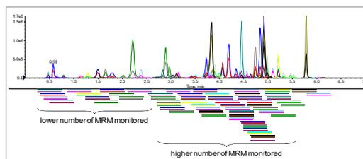
**Figure 2.** The *Scheduled MRM™* Algorithm uses the knowledge of the elution of each analyte to monitor MRM transitions only in a short retention time window. This allows many more MRM transitions to be monitored in a single LC run, while maintaining maximized dwell times and optimized cycle time.
