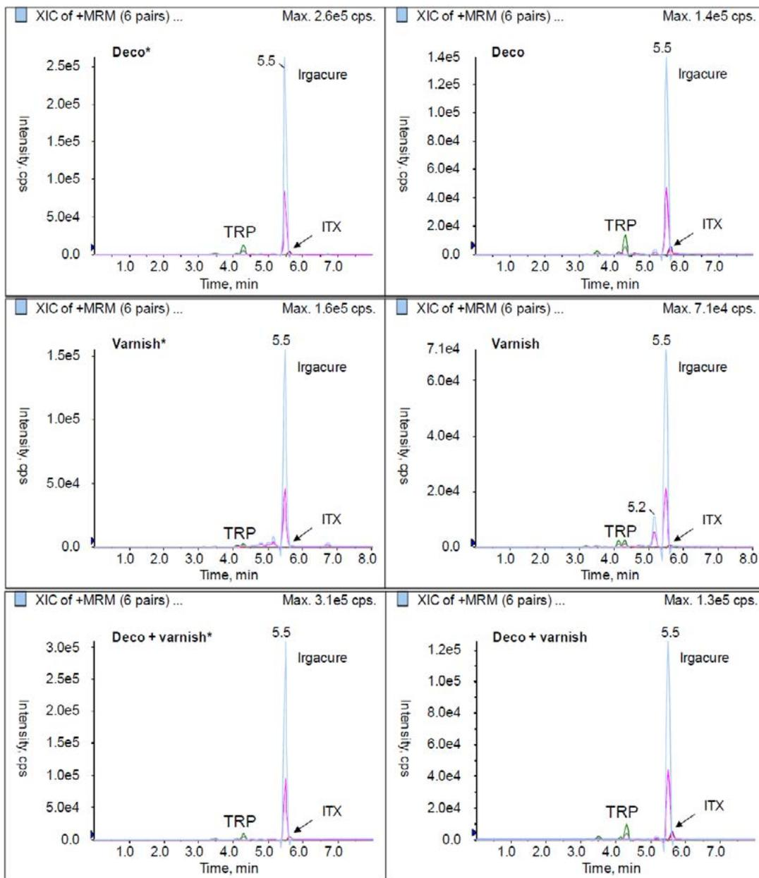
Figure 6. Sample Preparation Recoveries. A comparison of food packaging samples extracted with acetonitrile and where the acetonitrile extract of the same sample had been evaporated to dryness and reconstituted in mobile phase\* (cap with decoration (top), cap sealed with varnish (middle), and cap with decoration and sealed with varnish (bottom)).
