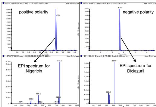
**Figure 4.** Example of an LC-MS/MS chromatogram from a 2 µg/L matrix matched calibration standard run in positive polarity with an EPI spectrum of Nigericin (left) and an LC-MS/MS chromatogram from the same sample run in negative polarity where a spectrum of Diclazuril has been automatically acquired
