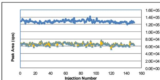
**Figure 5.** This graph shows the peak areas of two pesticides, Flutolanil (bottom) and Tricyclazole (top), which elute at different times during the run. It shows that the robustness is excellent with no deterioration in response even after 150 injections of a crude spice extract.
