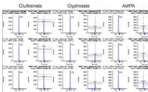
**Figure 5.** Triplicate analysis of polar pesticides in a spiked water sample at 0.1  $\mu$ g/L (injection volume of 10  $\mu$ L), ion ratios for compound identification were calculated automatically in MultiQuant<sup>™</sup> software version 3.0
