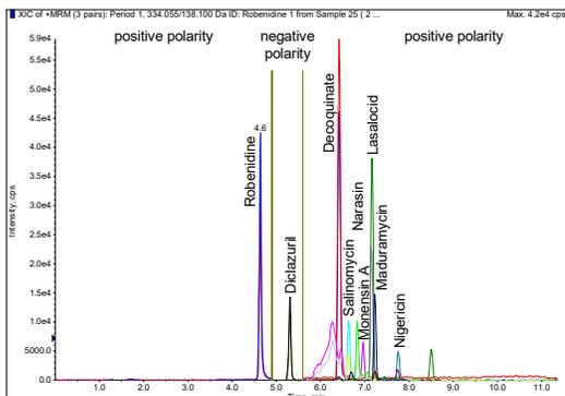
**Figure 2.** Example of an LC-MS/MS chromatogram from a milk matrix matched calibration standard (concentration of coccidiostats ranging from 2 to 10  $\mu\text{g}/\text{kg}$ ) prepared and analyzed using the new approach
