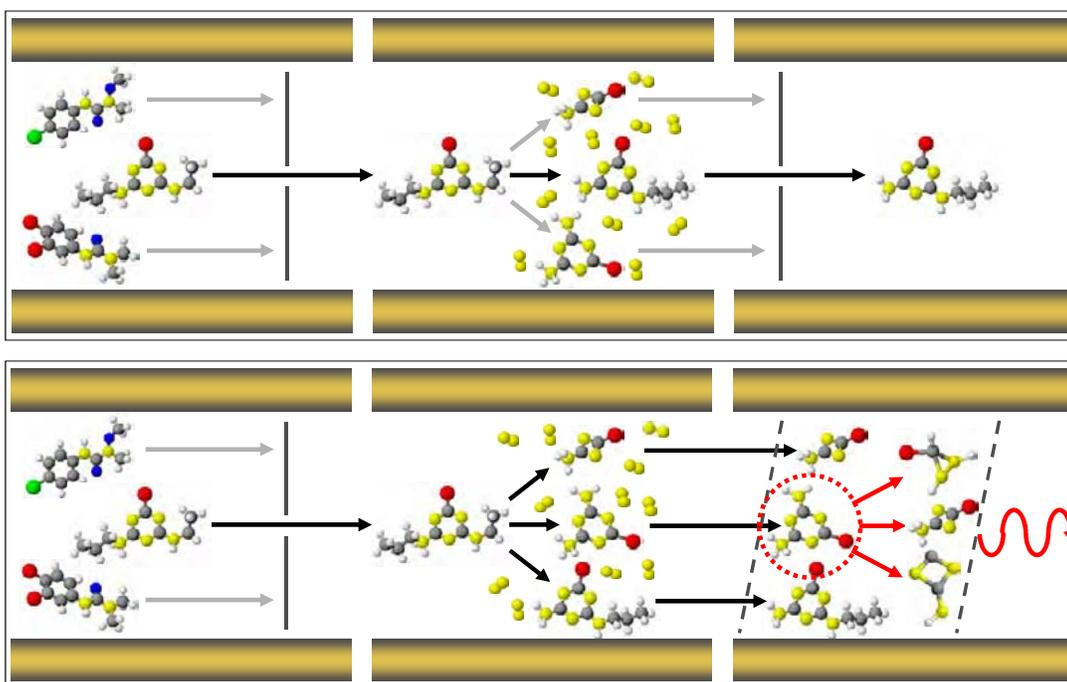
**Figure 1.** Operation of a QTRAP<sup>®</sup> system in MRM (top) and MRM<sup>3</sup> (bottom) modes
