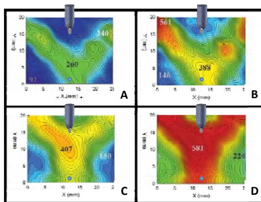
**Figure 1.** Temperature maps of the spray region of the traditional Turbo V<sup>™</sup> source (top) and the new IonDrive<sup>™</sup> Turbo V source (bottom). A and C show the source operated at 500°C and B and D at 700°C with Gas 2 set to 70 psi.
