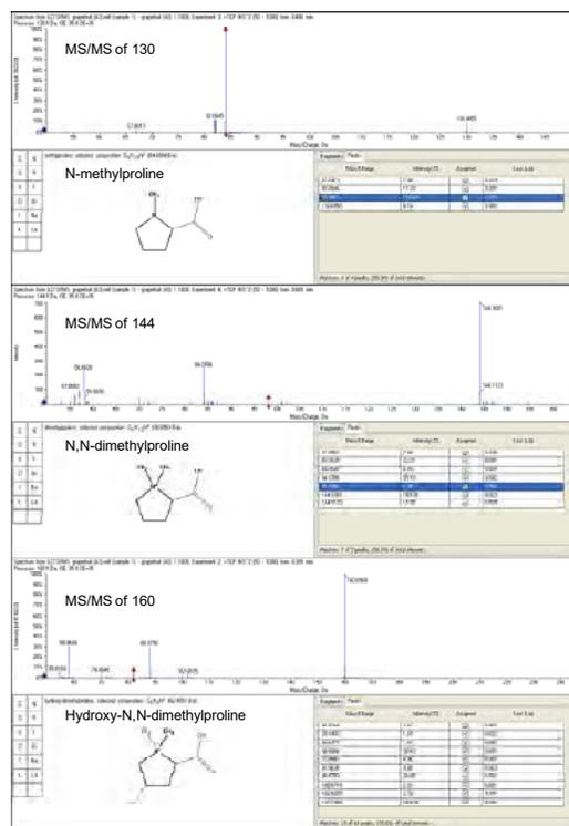
**Figure 7.** MS/MS fragment ion prediction for N-methylproline, N,N-dimethylproline, hydroxy-N,N-dimethylproline, 100% of MS/MS ions are explainable supporting the tentative identification in citrus fruits
