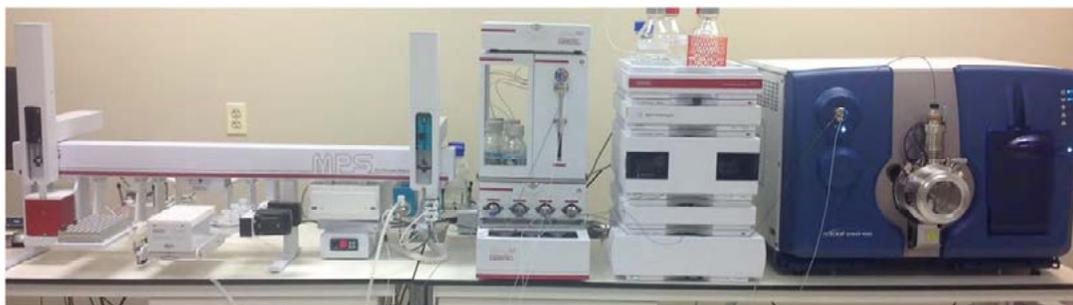
Figure 2. GERSTEL MPS 2XL with SPE<sup>XOS</sup> coupled to an QTRAP<sup>®</sup> 4500 system
