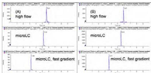
Figure 2. Comparison of high flow vs. microLC using a 1 ppm protein spike in white wine. A milk peptide is shown on the left (A) and an egg peptide is shown on the right (B).
