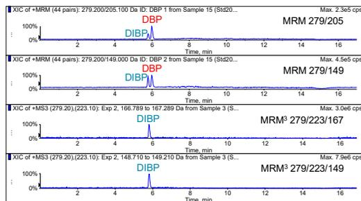
Figure 4. Differentiation of DIBP and DBP using the different fragmentation pattern in MRM<sup>3</sup> mode in comparison to MRM mode
