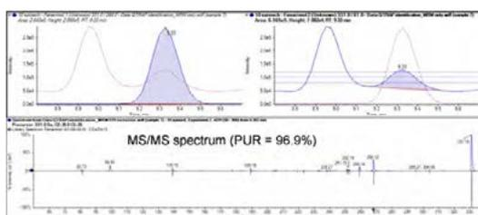
**Figure 8.** Detection of Fenarimol in spiked spinach: the MRM ratio was slightly out of the 30% tolerance due to high background and a closely eluting interfering matrix peak, but MS/MS library searching confirmed the presence of the detected pesticide.
