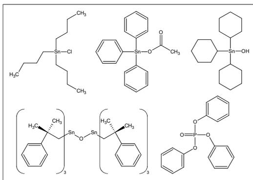
**Figure 1.** Target organotin compounds: TBT chloride, fentin acetate, cyhexatin, fenbutatin oxide, and internal standard triphenyl phosphate (top left to bottom right)
