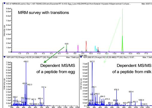
**Figure 3a.** MIDAS™ workflow for the detection of allergens in pasta. Analysis of an extract from pasta spiked at 100 ppm with egg and milk allergens. The top pane shows the total ion chromatogram for all MRM transitions; the bottom left pane shows the QTRAP® MS/MS spectrum which has been automatically generated by an egg peptide, and the bottom right pane is the spectrum generated by a milk peptide
