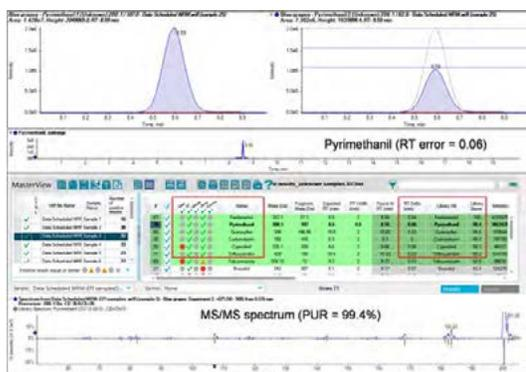
**Figure 10.** Fenhexamid, Pyrimethanil, Quinoxifen, and Trifloxystrobin were identified based on MRM ratios and quantified in a grapes sample, the MRM ratio of Pyrimethanil were slightly outside the 30% tolerance (top), however, second analysis using MS/MS library searching confirmed the presence of Pyrimethanil (bottom)
