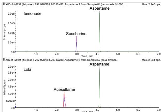
**Figure 3.** Chromatograms obtained from a 1000 dilution of a lemonade sample (top) and of a cola sample (bottom). The two sweeteners detected corresponded to those listed on the drink's label.
