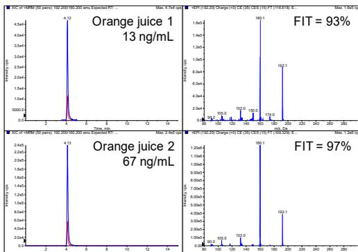
**Figure 6.** Identification of Carbendazim in two orange juice samples using MS/MS library searching, the samples were injected directly after 5x dilution, FIT values above 90% clearly confirm the identity of Carbendazim
