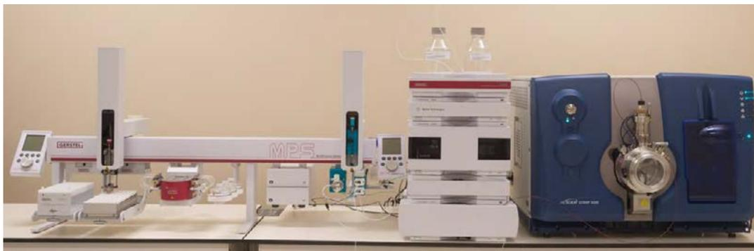
Figure 1. GERSTEL MPS 2XL with DPX option coupled to an QTRAP<sup>®</sup> 4500 system
