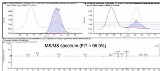
**Figure 2.** Detection of Fenarimol in spiked spinach: the MRM ratio was slightly out of the 30% tolerance due to high background and a closely eluting interfering matrix peak, but MS/MS library searching confirmed the presence of the detected pesticide.
