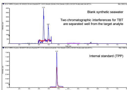
**Figure 3.** Blank synthetic seawater, two chromatographic interferences for TBT are separated well from the target analyte (top) and internal standard (bottom)
