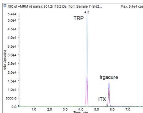
Figure 4. Chromatographic Separation. 10 µL injection of migrant standards in initial mobile phase.
