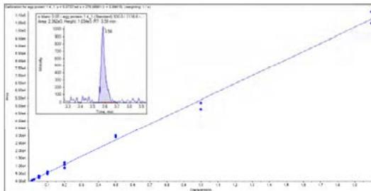
**Figure 3.** Calibration line from a peptide from egg which had been spiked into a sauvignon blanc wine (0.01 to 2 ppm) and chromatogram of the 50 ppb spike sample. The linearity is provided without the use of any internal standards.
