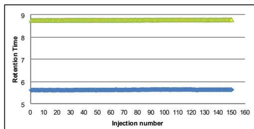
**Figure 4.** In this graph, retention time of two pesticides, Flutolanil (top) and Tricyclazole (bottom) were plotted against the injection number. The graph shows that the retention times obtained are rock solid with little or no variation between injections, confirming the low dead volume of the system and that fast equilibration times are possible.
