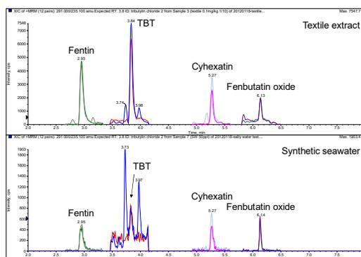
**Figure 5.** Textile material spiked with 0.1 mg/kg and diluted 10x after extraction (top) and synthetic seawater spiked at 50 ng/L and analyzed by direct injection (50 µL)
