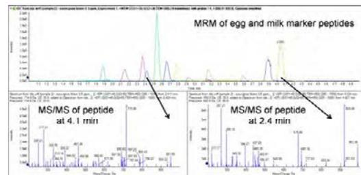
**Figure 5.** Micro flow LC-MS/MS analysis of 0.5 ppm spike of egg and milk proteins into a sauvignon blanc sample analyzed using the MIDAS™ workflow. The top pane shows the extracted ion chromatogram for the peptides of milk and egg and the bottom two panes show examples of MS/MS spectra for target peptides
