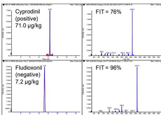
**Figure 7.** Identification of Cyprodinil and Fludioxonil in a raspberry sample using MS/MS library searching, the samples were injected after QuEChERS extraction and 5x dilution, MS/MS spectra were acquired in positive polarity and negative polarity
