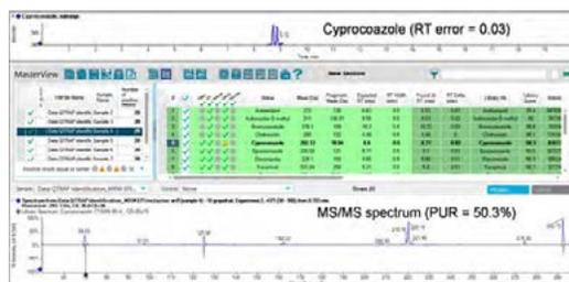
**Figure 9.** Detection of Cyproconazole in grapefruit: the MS/MS library search resulted in a PUR value of 50.3% only, however, review of spectra revealed in isobaric matrix interference, the MRM ratio error of 6.9% further confirmed the presence of the pesticide.
