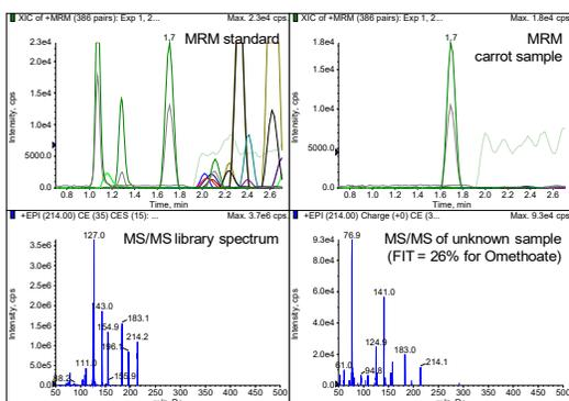
**Figure 8.** False positive finding identified by MS/MS library searching, standard and carrot sample have identical retention times of 1.7 min and MRM ratio of 0.6 but MS/MS spectra differ and the search results clearly prove the false positive
