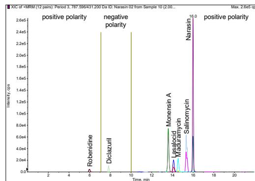
**Figure 1.** Example of an LC-MS/MS chromatogram from a milk matrix matched calibration standard (concentration of coccidiostats ranging from 2 to 10  $\mu$ g/kg) prepared and analyzed using the conventional approach
