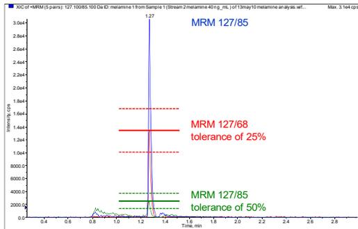
**Figure 6.** Chromatogram of melamine spiked into milk with MRM ratio tolerances for compound identification as defined by the European guideline 2002/657/EC<sup>7</sup>
