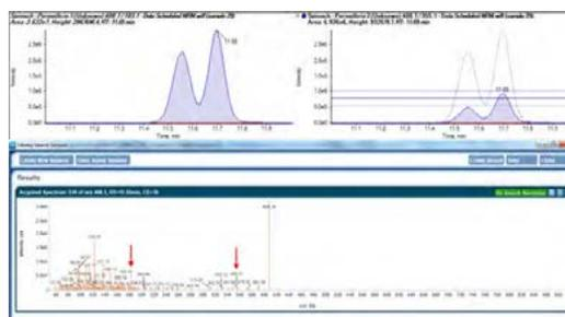
**Figure 12.** Permethrin was detected in the spinach sample at a high concentration of 1060 µg/kg, the identification using MRM ratio was positive but the MS/MS library searching indicates strong matrix interferences, manual searching in LibraryView™ software confirms the presence of both characteristic ions in the MS/MS spectrum, further confidence is gained through the presence of characteristic isomers in the LC profile
