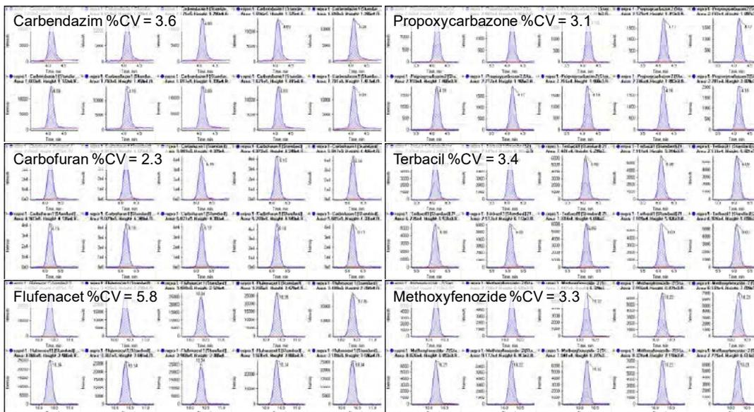
**Figure 2.** Repeat injections of pesticides at a concentration of 1 ng/mL detected in positive (left) and negative (right) polarity in a single run using *Scheduled MRM™* and fast polarity switching (Carbendazim and Propoxycarbazone at 4.1 min, Carbofuran and Terbacil at 6.1 min, and Flufenacet and Methoxyfenozide at 10.3 min)
