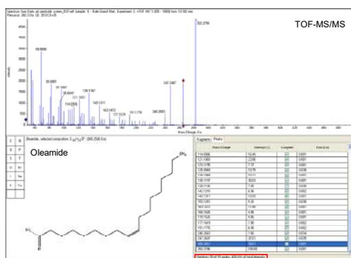
**Figure 10.** MS/MS fragment ion prediction for Oleamide, 100% of MS/MS ions are explainable by the structure of Oleamide
