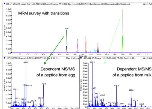
**Figure 3b.** MIDAS™ workflow for the detection of allergens in bread. Analysis of an extract from bread spiked at 100 ppm with egg and milk allergens. The top pane shows the total ion chromatogram for all MRM transitions; the bottom left pane shows the QTRAP® MS/MS spectrum which has been automatically generated by an egg peptide, and the bottom right pane is the spectrum generated by a milk peptide
