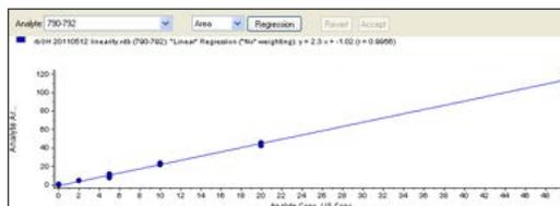
Figure 3. Calibration line for extracts of milk samples spiked with rbST at different levels. The calibration line is from the MRM<sup>3</sup> experiment 913.2/774.0/791.0
