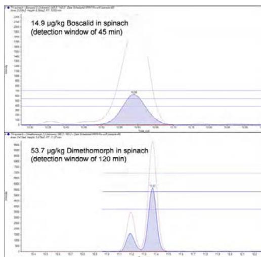
**Figure 7.** Examples of using the Flexible Window Width in a *Scheduled MRM™ Pro* method: the window for Boscalid was set to 45 sec and Dimethomorph was detected using a wider window to detect both isomers together
