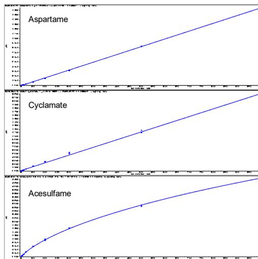
**Figure 5.** Examples of calibration curves for three commonly detected artificial sweeteners [Aspartame (top), Cyclamate (middle) and Acesulfame (bottom)], as it can be seen some compounds produce a non linear response over the range from 1 to 1000 ppb,
