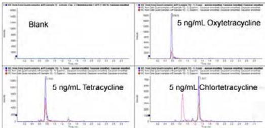
**Figure 2.** Sensitivity of a 5 ng/mL standard of tetracyclines (injection volume of 10  $\mu\text{L}$ )
