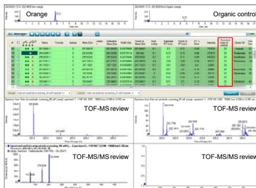
**Figure 8.** Identification of Imazalil and Thiabendazole using a non-targeted sample-control-comparison and MS/MS library searching, the software automatically reports all ions which are 20 times higher in the sample versus the organic control
