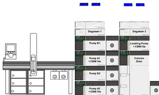
Figure 1. SCIEX MPX™-2 SP High Throughput system: configuration and module arrangement
