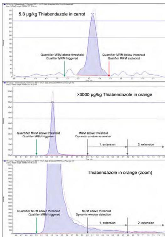
**Figure 8.** Examples of MRM-triggered MRM and Dynamic Window Extension: the qualifier MRM transition is automatically triggered when the quantifier MRM transitions exceeds the threshold set in the *Scheduled MRM™* Pro method, the detection window is automatically extended if the MRM signal is above the threshold at the end of the detection window
