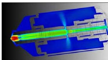
**Figure 2.** Computed gas flow model of the dual stage QJet<sup>™</sup> ion guide
