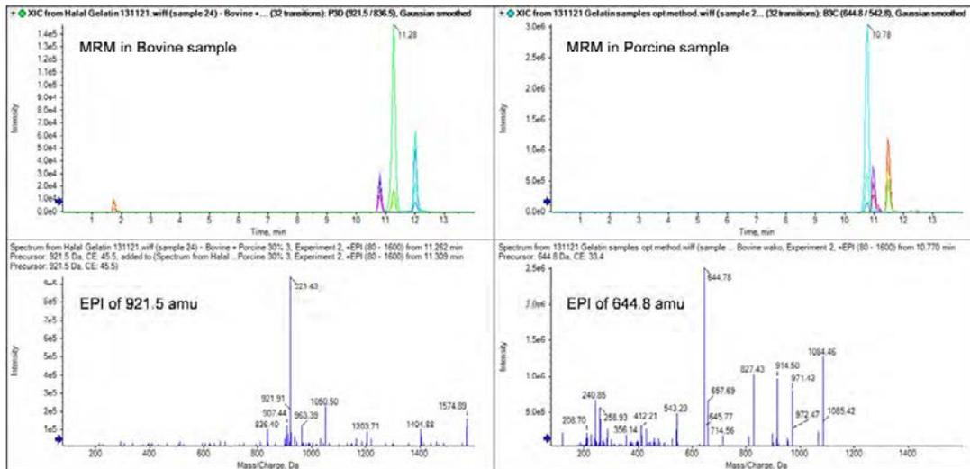
**Figure 3.** Comparison of a tryptic digest of a porcine (left) and a bovine (right) gelatin standard, MRM transitions were used to automatically acquire full scan EPI spectra for identification of the gelatin marker
