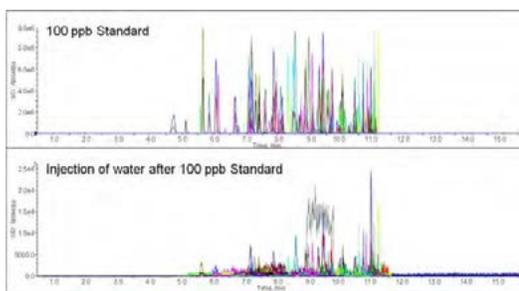
**Figure 2.** The top pane shows a 100 ppb calibration standard injected using the micro flow LC MS/MS set-up. The bottom pane shows water injected directly after this standard showing very low carryover.
