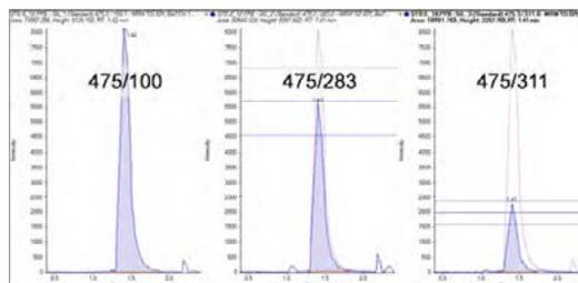
Figure 2. MRM transitions of Sildenafil at a concentration of 10 ng/mL, the MRM ratio was automatically calculated in MultiQuant<sup>™</sup> software (Sildenafil 2: 0.686 ± 20%, Sildenafil 3: 0.210 ± 25%)
