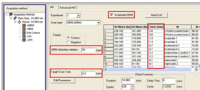
**Figure 3.** Acquisition method interface for *Scheduled MRM™*, in addition to traditional MRM parameters, the user provides retention times of all analytes, an MRM detection window, and a Target scan time. The software then automatically designs and optimizes the *Scheduled MRM™* acquisition method.
