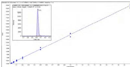
**Figure 4.** Calibration line from a peptide from milk which had been spiked into a sauvignon blanc wine (0.01 to 2 ppm) and chromatogram of the 50 ppb spike sample. The linearity is provided without the use of any internal standards.
