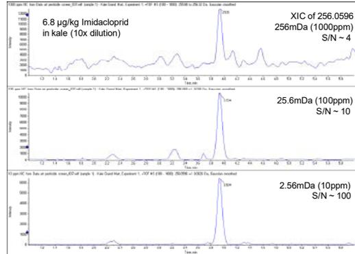
**Figure 2.** Increasing selectivity and S/N using narrow extracted ion chromatograms (XIC)
