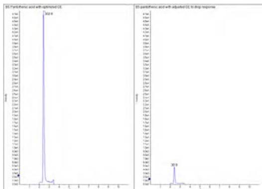
**Figure 3.** The effect of changing the collision energy on the response of vitamin B5
