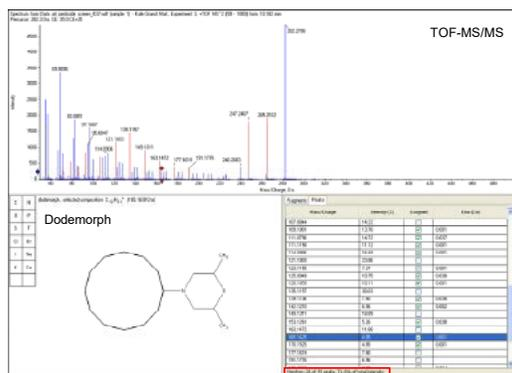
**Figure 11.** MS/MS fragment ion prediction for Dodemorph, many MS/MS ions cannot be explained by the structure suggesting that Dodemorph was not present in the kale sample
