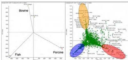
**Figure 1.** MarkerView<sup>™</sup> software was used to identify characteristic markers for gelatin speciation, PCA Scores plot for bovine, porcine and fish (left) and PCA Loadings showing characteristic markers (right)
