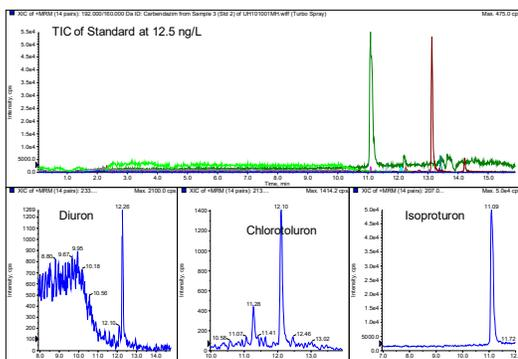
Figure 5a. 12.5 ng/L standard in positive polarity
