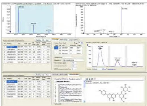
**Figure 6b.** Tentative identification of a marker ion characteristic for grapefruit (603 at 4.4 min) as naringin (naringoside) based on empirical formula finding and automatic online database searching
