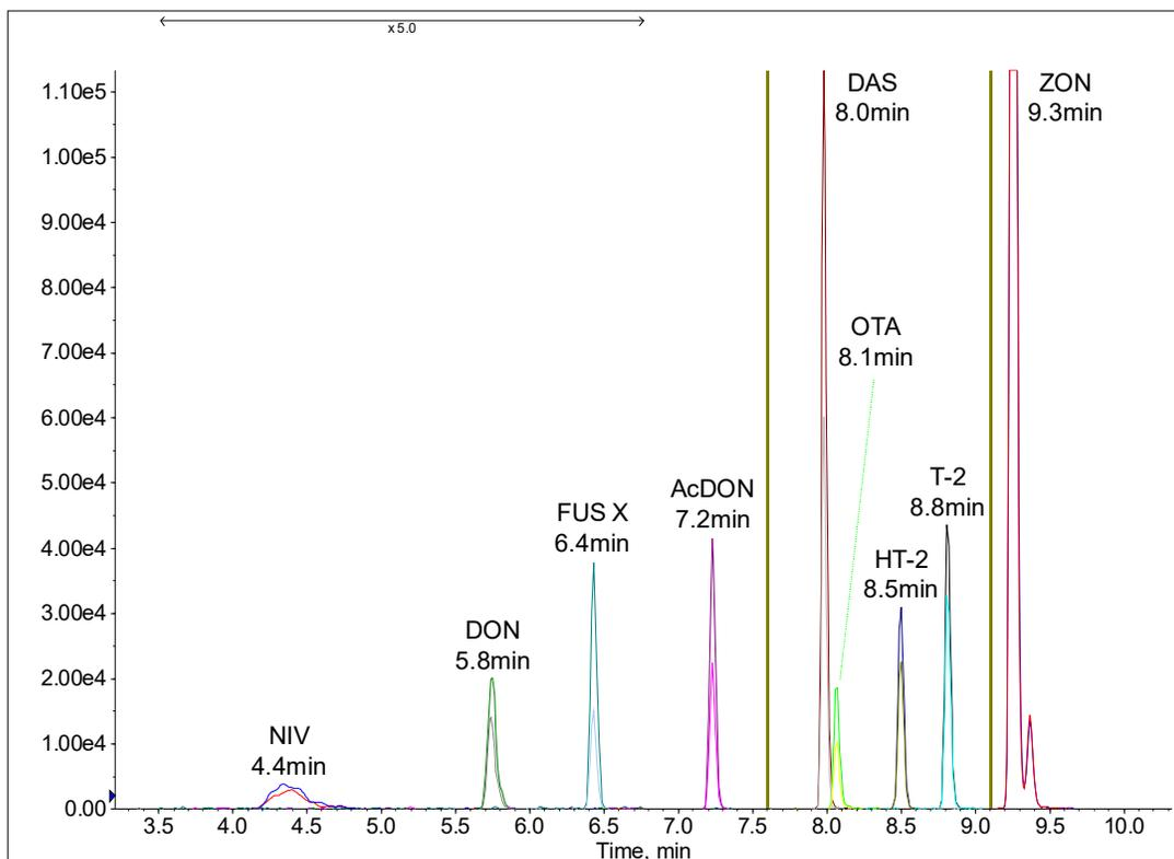
**Figure 3.** Mycotoxin standard analyzed using LC-MS/MS in MRM
