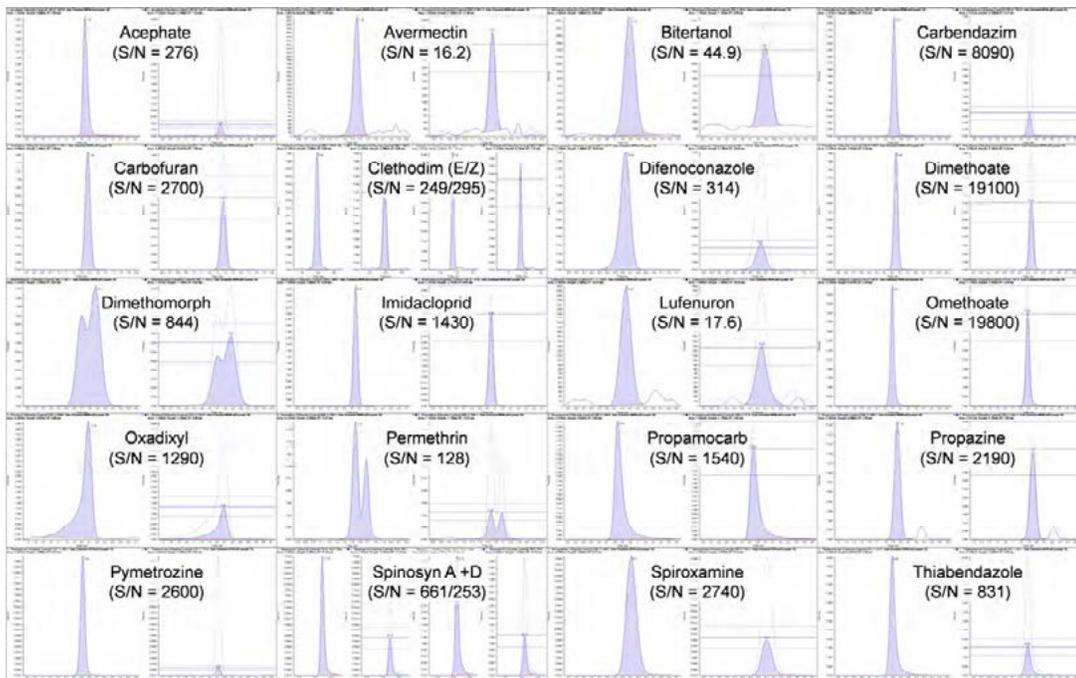
**Figure 4.** Quantifier and qualifier MRM transitions of selected pesticides with S/N at a concentration of 1 ng/mL, the MRM ratio tolerance of 30% is displayed in the MultiQuant™ software peak review (SANCO/12571/2013)
