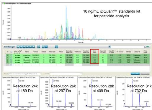
**Figure 1.** Resolution and mass accuracy across the mass range for selected pesticides of the iDQuant™ standards kit
