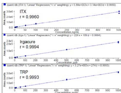
Figure 3. Quantitation Curves. Calibration lines obtained from ITX, Irgacure and TRP with r values > 0.996 (no internal standard used).
