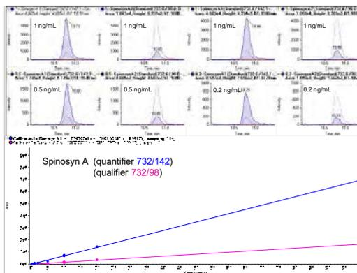
Figure 4c. Calibration lines of the quantifier and qualifier MRM transition of Spinosyn A from 0.1 to 100 ng/mL.
