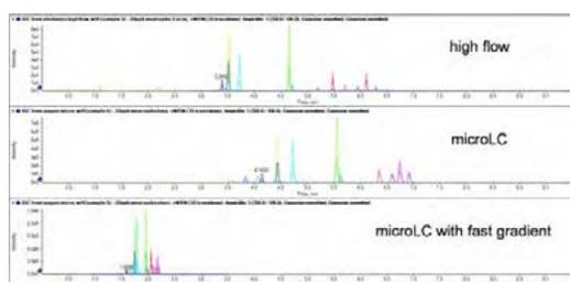
**Figure 3.** Comparison of meat sample spiked at 20  $\mu$ g/kg and analyzed by traditional high flow LC and micro flow LC-MS/MS. In this example analysis time was decreased from 10 min to 3.5 min using micro flow LC and by speeding up the gradient. In all methods peak widths at the base were 3 seconds or less.
