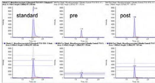
**Figure 4.** Chromatograms of standard at 10 ng/mL in comparison to the pre-extraction and post-extraction spike of milk at 10 ng/mL (the quantifier ion results are shown on the top row and the qualifier ion on the bottom row)
