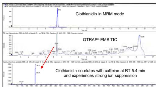
**Figure 8.** Monitoring of matrix effects by simultaneous acquisition of target MRM transitions and EMS scans, the strong ion suppression observed for Clothianidin can be explained by co-elution with caffeine at a much higher concentration
