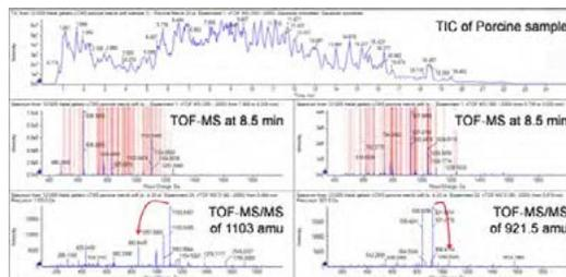
**Figure 2.** TOF-MS and TOF-MS/MS data of two selected marker compounds for porcine, TripleTOF<sup>®</sup> data was used to develop the MRM method
