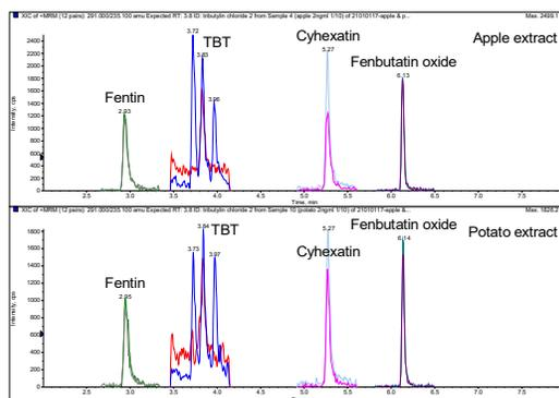
**Figure 4.** Apple (top) and potato (bottom) sample spiked at 2 µg/kg and diluted 10x after extraction
