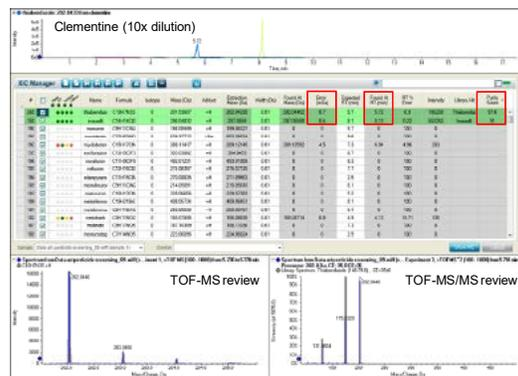
**Figure 3.** Identification of Imazalil and Thiabendazole in a clementine sample, retention time, mass accuracy, isotopic pattern, and MS/MS library match were reported automatically and visualized using 'traffic lights'
