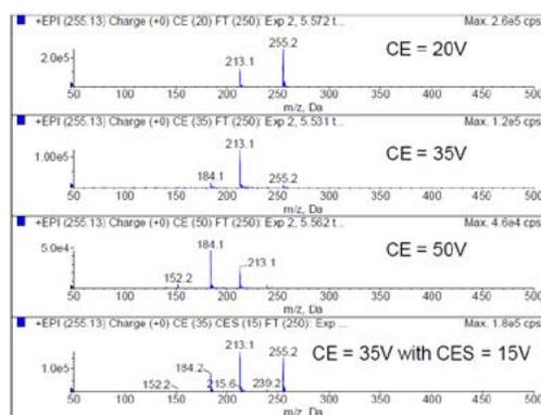
**Figure 2. Optimizing Collision Energies.** An example of the effect of collision energy on the EPI spectra of a migrant standard used for generating library data (10 ng/mL ITX standard).
