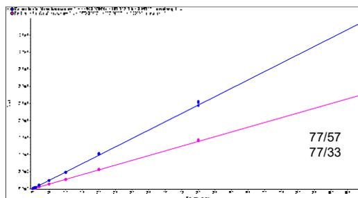
Figure 3. Calibration lines (0.1 to 100 ng/mL) for sodium fluoroacetate
