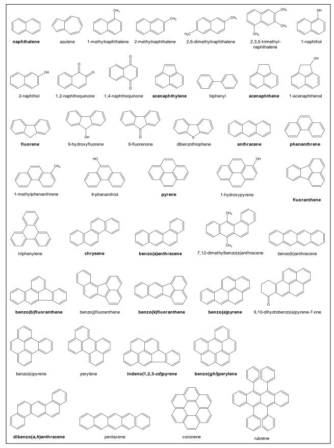
Figure 1. Structures of targeted PAH, alkylated derivatives, and photo-degradation products (Compounds in bold are the 16 EPA priority PAH.)
