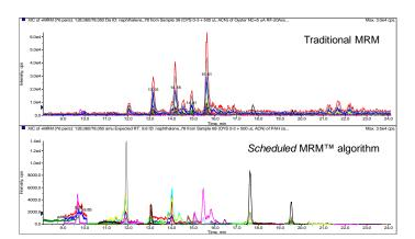
Figure 5. Analysis of an oyster extract using traditional MRM and the *Scheduled* MRM<sup>™</sup> algorithm
