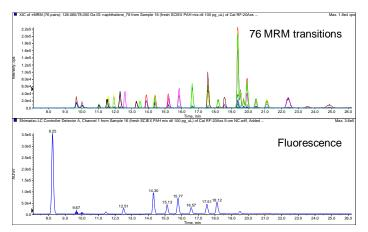
Figure 2: LC-MS/MS (top) and LC-FLD (bottom) analysis of PAH, alkylated derivatives, and photo-degradation products
