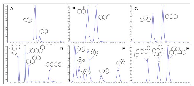
Figure 3. Separation of critical isomers using the developed LC method
