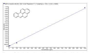
Figure 4. Calibration line of benzo(a)pyrene using triplicate injections into LC-MS/MS with APCI
