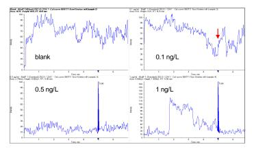
Figure 7. Parts-per-trillion level (ppt) detection of benzo(a)pyrene in drinking water. The direct injection of 1 mL into LC-MS/MS allowed quantitation with an LOD of less than 1 ng/L using the QTRAP<sup>®</sup> 5500 system.
