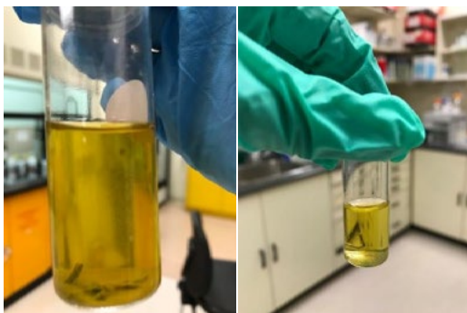
Figure 1: Variability in Matrix. Flower extract after winterization (left). Flower extract after two rounds of winterization at -20°C (right).
