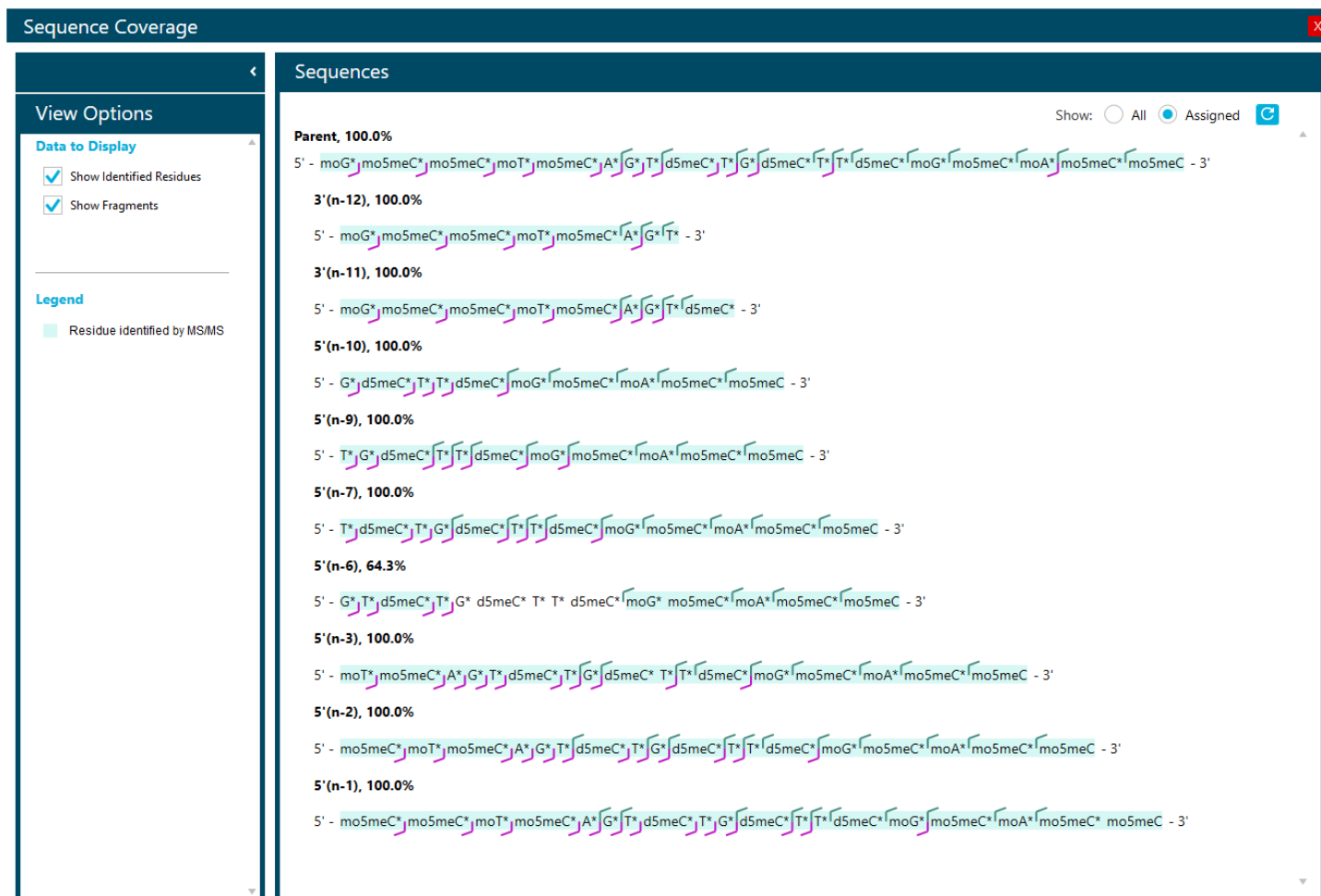
Figure 8. Summary of sequence coverage for the FLP (Parent) and all spiked-in metabolites. Sequence coverage is determined using fragments assigned in all identified charge states of a metabolite that MS/MS spectra were acquired for. A, c, d, w and y terminal ions were considered and 1 water or base loss was allowed. A minimum S/N ratio of 50 was used.
