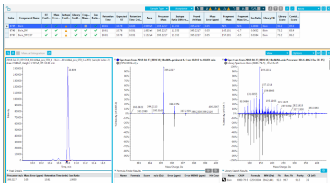
Figure 1. Results for a couscous sample adulterated with bixin (precursor mass, isotope distribution and MS/MS spectra).
