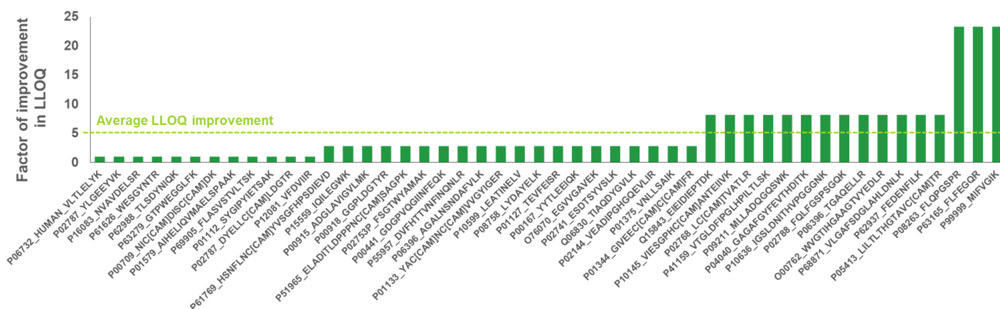
Figure 1. Factor of improvement in LLOQ for peptide quantification with Zeno MRM HR compared to MRM HR . On average, a 5-fold improvement in LLOQ for peptide quantification was observed with Zeno MRM HR in comparison to standard MRM HR .
