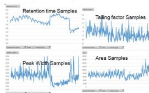
Figure 5. Reproducibility data for glyphosate IS. NofaLab method for food samples, tested over 1000 injections of extracts from fruit/veg, seeds, veg oil/fat, grains, herbs/spices, meat/fish, animal oil/fat, eggs/egg products, milk/milk products and other fatty acids.
