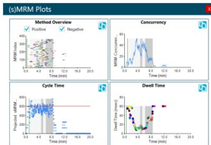
Figure 2. Scheduled MRM algorithm plots in SCIEX OS software. The scheduled MRM algorithm enables the analysis of hundreds of compounds in a single analysis with high quantitative accuracy. Each MRM transition is acquired during a short retention time window around its known elution time. This allows more MRM transitions to be monitored in a single LC run, while still maintaining maximized dwell times and optimized cycle times. 6 In SCIEX OS software, new visualization plots are available to help with method development and improve overall data quality.
