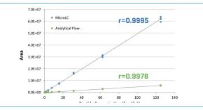
Calibration curves are shown for a synthetic peptide [VGNEIQYVALR] in diluted crashed plasma using microflow LC-MS at 3  $\mu$ L/min and analytical flow LC-MS at 500  $\mu$ L/min. LLOQ with microflow LC was 8x lower than what could be achieved with analytical flow LC-MS, and linearity was excellent for both flow rates.
