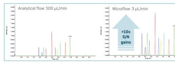
Peptide mix separation (500 µL/min) is shown with a 2.6 µm C18 3 x 50 mm column and no matrix.
