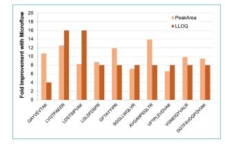
LLOQ gains and peak area improvements are shown for 10 synthetic peptides in diluted crashed plasma using microflow LC-MS at 3  $\mu$ L/min vs. analytical flow LC-MS at 500  $\mu$ L/min.
