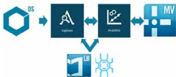
Figure 2. Workflow diagram. Data was both acquired and processed using SCIEX OS software. MS/MS was interpreted using both Explorer and Analytics, library searching was performed using the Library View and ChemSpider.
